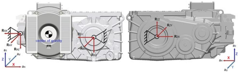
Fig. 3.13. Fixing scheme for load modes I, II, III.
