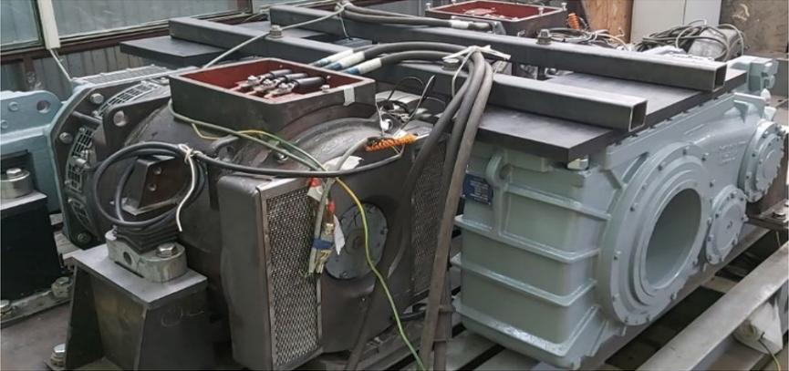
Fig. 5.16. Physical testbench of MGU under the mutual load control.
