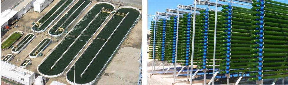
Figure 1.4. Open (left) and closed (right) systems for microalgae production (Copyright: Green Prophet and Varicon Aqua).
