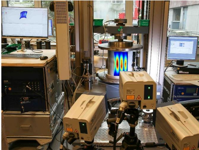
Fig. 2.6. Typical VCT test set up.
