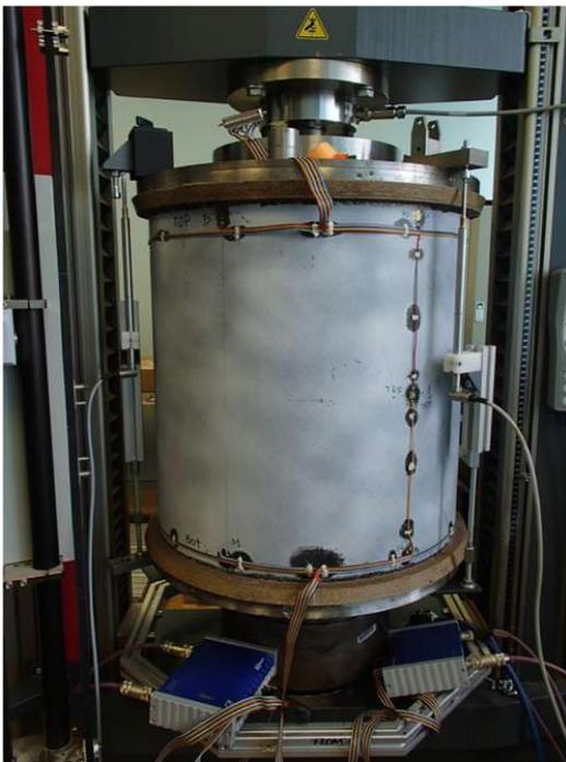
Fig. 4. Experimental test setup for compressive loading on cylindrical shells.
