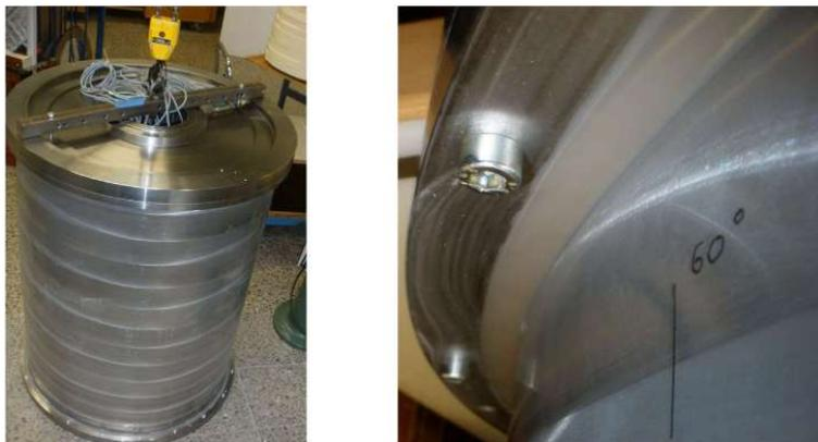
(a) Overview of the potted cylindrical shell. (b) Detail of the upper steel ring.
