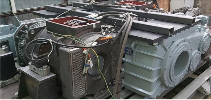
Fig. 5.8. Physical testbench of MGU under the mutual load control.
