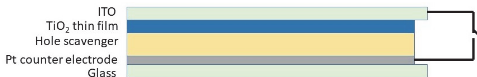
Fig. 3.13. Photoelectron device schematic
