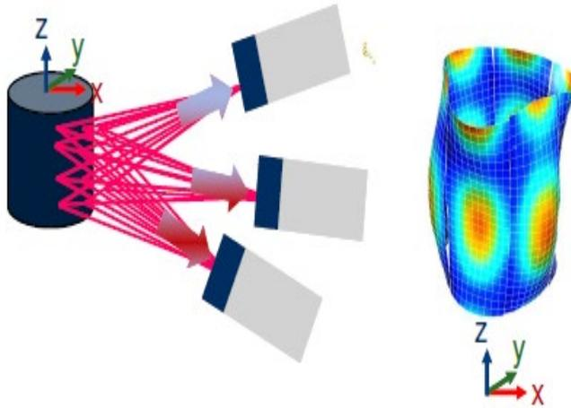
Fig. 2.8. Working principle of PSV-500-3D (Polytec, Polytec PSV-E-500 Operating Instructions Manual, 2016).
