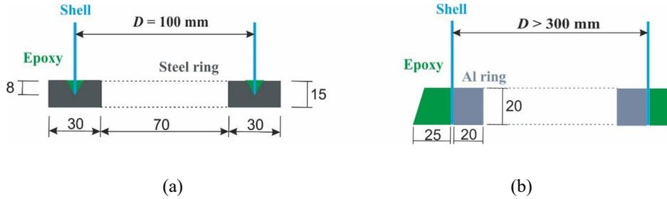
Fig. 2.5. Schematic of the mounting of cylinders: (a) in the groove of a steel ring; (b) potting onto plates of the test machine. Dimensions in the figure are given in mm.
