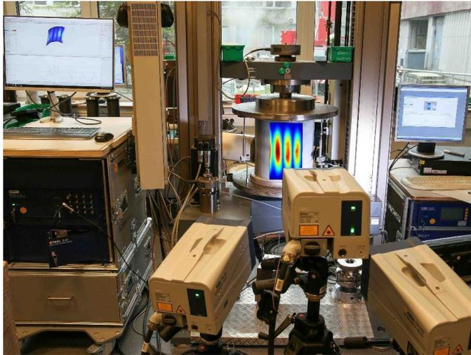
Fig. 2.6. Typical VCT test set up.
