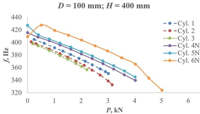
Fig. 2.15. Anomaly at the initial testing stage.
