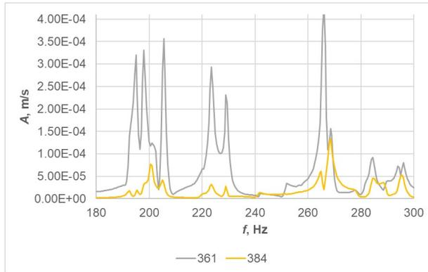
Fig. 2.13. Frequency response with bad and good measurement points.
