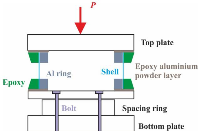
Fig. 2.4. Schematic of the setup for compression tests of cylinders, testing using the shimming of the plate.
