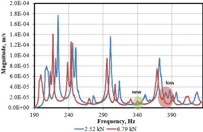
Fig. 2.11. Frequency response, example loss and new eigen frequency.
