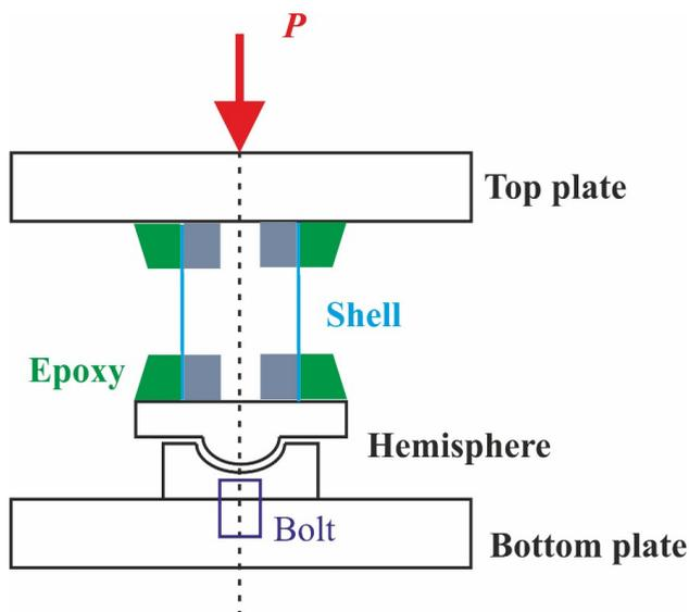
Fig. 2.2. Schematic of the setup for compression tests of cylinders, testing using a hemispherical joint.
