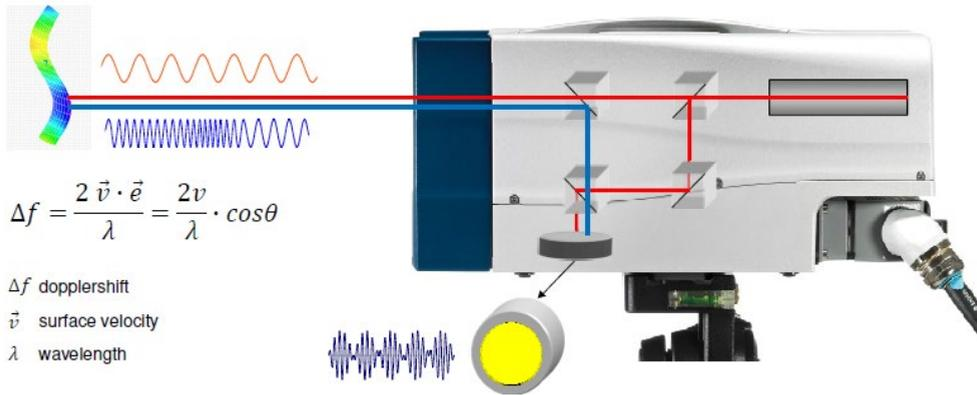
Fig. 2.7. Technological background (Polytec, Polytec Scanning Vibrometer, Theory Manual. PSV, PSV-3D, MSA/MSV, as of Software 8.5, 2001).
