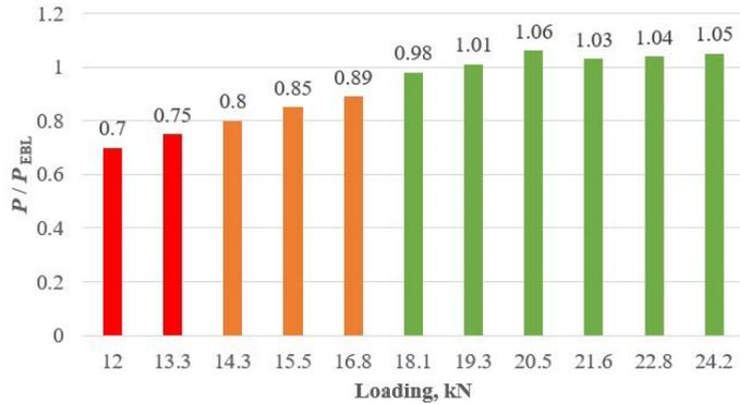
Fig. 2.14. Buckling load prediction using the VCT approach for different loading ranges.
