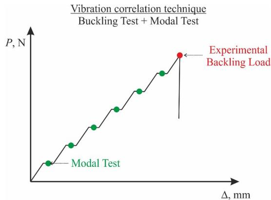
Fig. 2.1. Experimental VCT testing – step loading.
