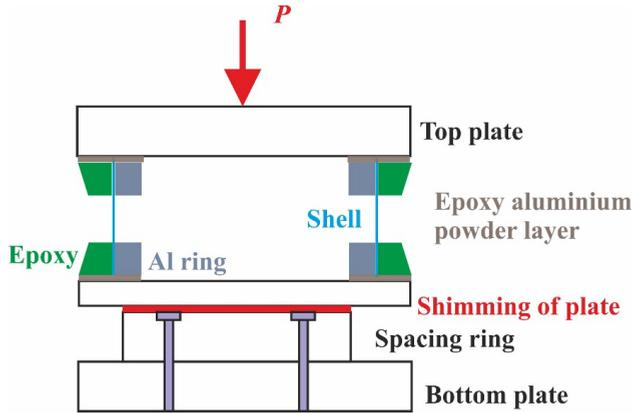
Fig. 2.3. Schematic of the setup for compression tests of cylinders, testing using the shimming of the plate.
