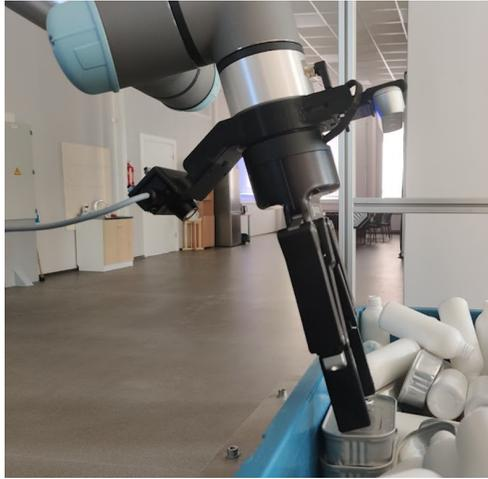
5.13. Fig. Sensors attached to the robotic arm.
