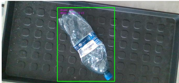
5.12. Fig. A bounding box from object detector and determined angle and width from the proposed approach.
