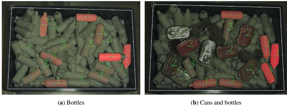
3.1. Fig. Different scenarios that include segmented objects with calculated grasp positions.
