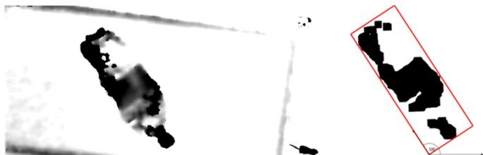
5.11. Fig. Full depth map and ROI after thresholding and calculating the angle.
