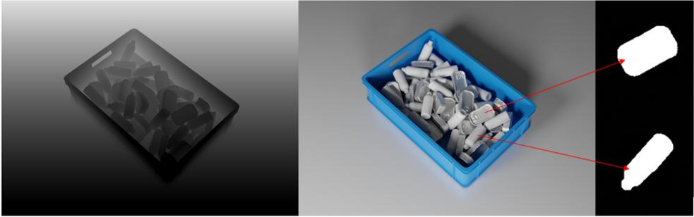
5.7. Fig. Scene including the plastic bottle- and the reconstructed metal can 3d models (middle) together with the corresponding depth image (left) and segmentation masks (right).
