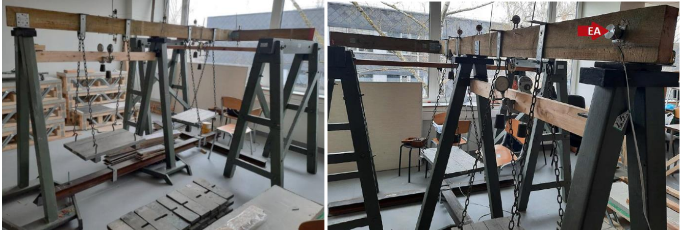
Figure 1. Stand of two timber beams connected at an angle of 90^\circ and electrodynamic actuators “EA”.
