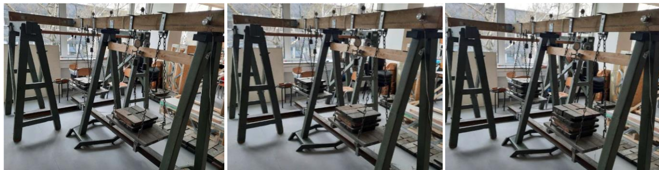
Figure 5. Load level of 120 kg (left), 180 kg (middle) and 240 kg (right) of the timber beams stand.
