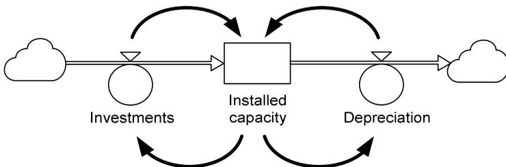
Fig.1.2. Elements of system dynamic model, blocks and flows
