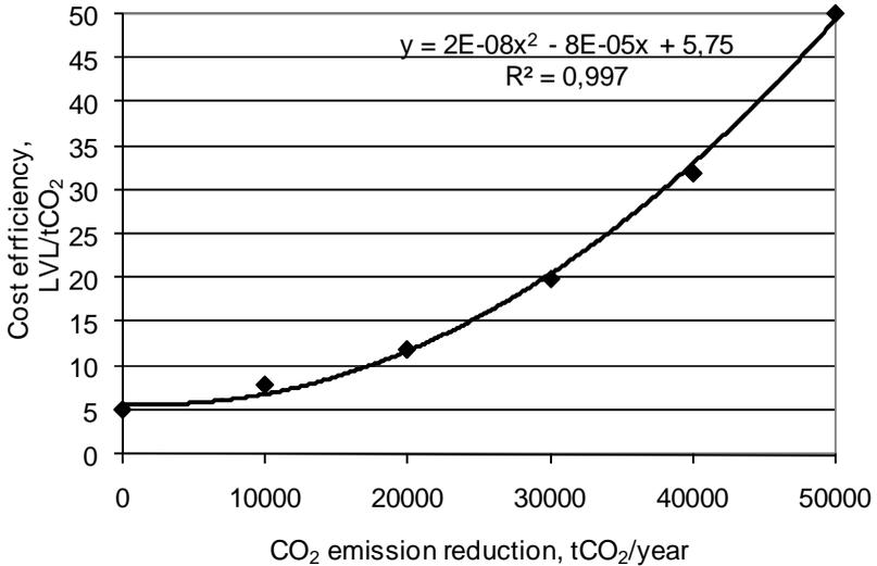
Fig.2.2. Relation between CO<sub>2</sub> emission reduction costs and CO<sub>2</sub> emission reduction
