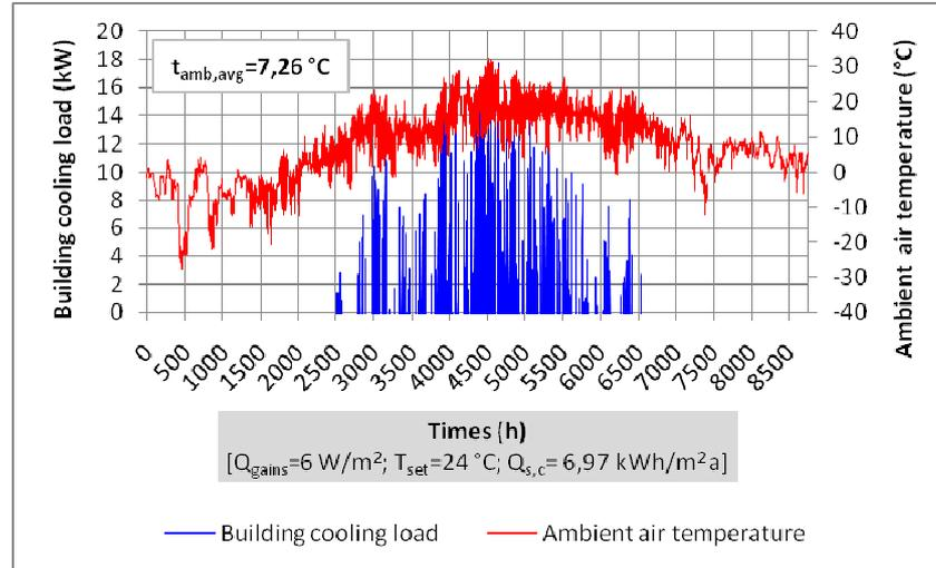
Fig. 2.1. The research target building's simulated cooling load and ambient air temperature fluctuations throughout the year
