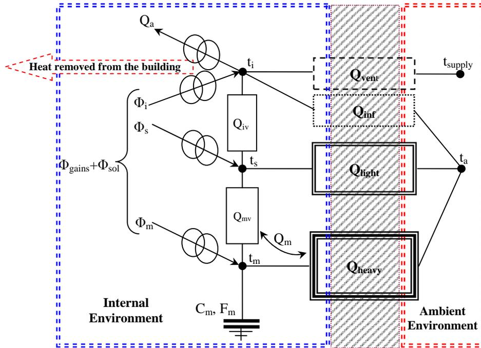
Fig. 1.1. Network nodes of the building dynamic cooling load calculation model “Cool”
