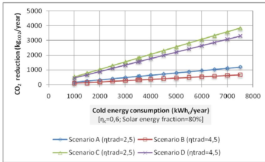
Fig. 4.5. CO<sub>2</sub> reduction depending on cooling energy consumption
