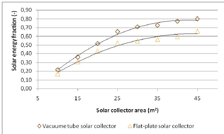
Fig. 4.3. Changes in solar energy supply depending on solar collector type and nominal area
