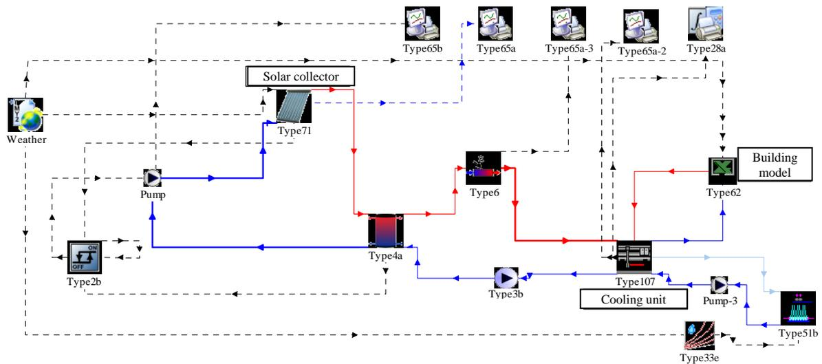
Fig. 4.2. Diagram of simulated solar cooling system in the environment of TRNSYS simulation program
