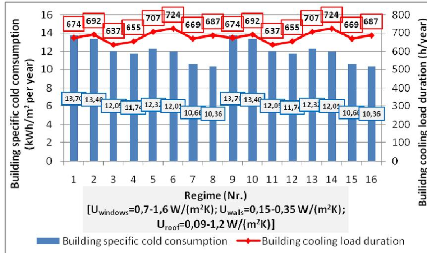
Fig. 2.3. The building's specific cooling consumption and building cooling load duration depending on the mode of the quantitative experiment
