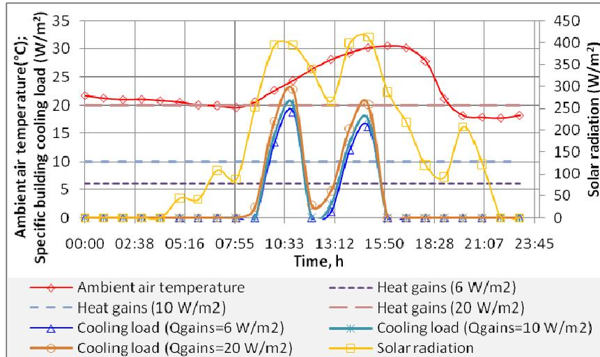
Fig. 2.2. Daily fluctuations of the research target building's simulated cooling load, ambient air temperature and solar radiation in July
