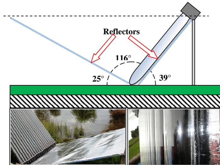
Fig. 3.3. Diagram of vacuum tube solar collector with reflectors and reflectors' location
