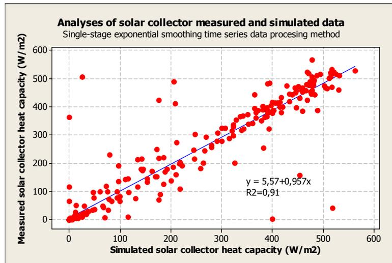
Fig. 3.5. Analyses of the measured and simulated data of solar collector heat capacity
