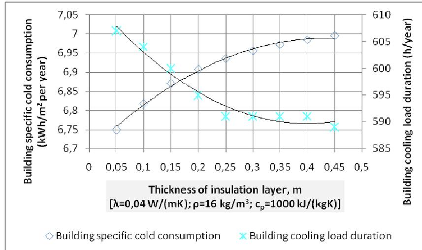
Fig. 2.5. Changes of building specific cooling consumption and building cooling load duration depending on thickness of heating insulation layer
