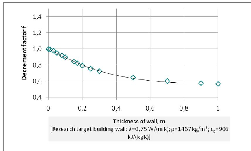
Fig. 2.7. Changes of temperature fluctuation amplitude decrement factor  $f$  depending on thickness of research target building wall
