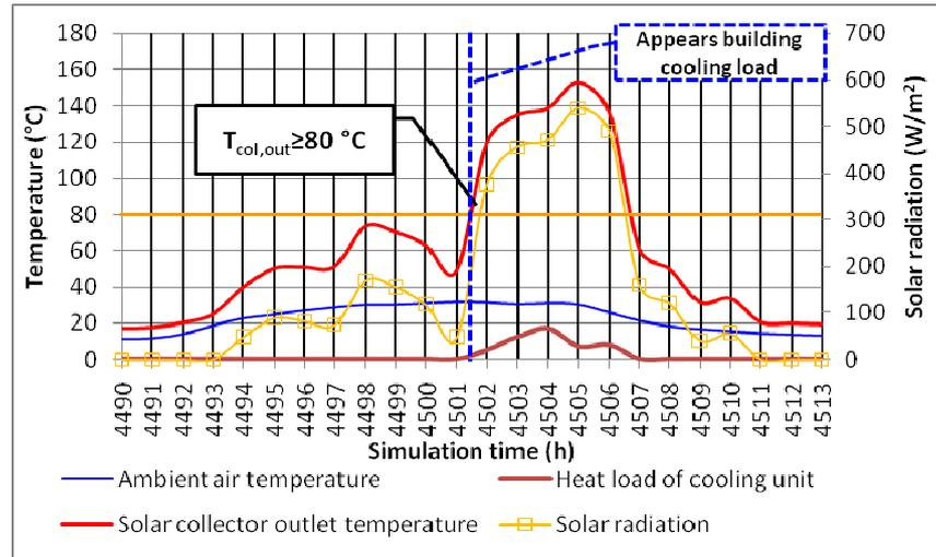
Fig. 4.4. Required changes in heating load of cooling device and supply temperature of solar collector (area 45 m<sup>2</sup>)
