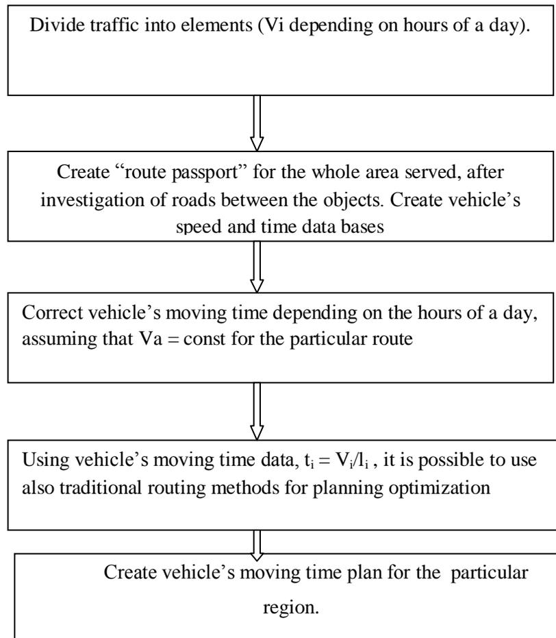
Figure 3.4. Vehicle's moving time planning scheme, using micro-elements standardization method.
