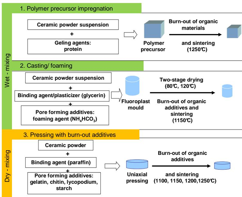
Fig. 1. Technologies of obtaining porous bioceramics
