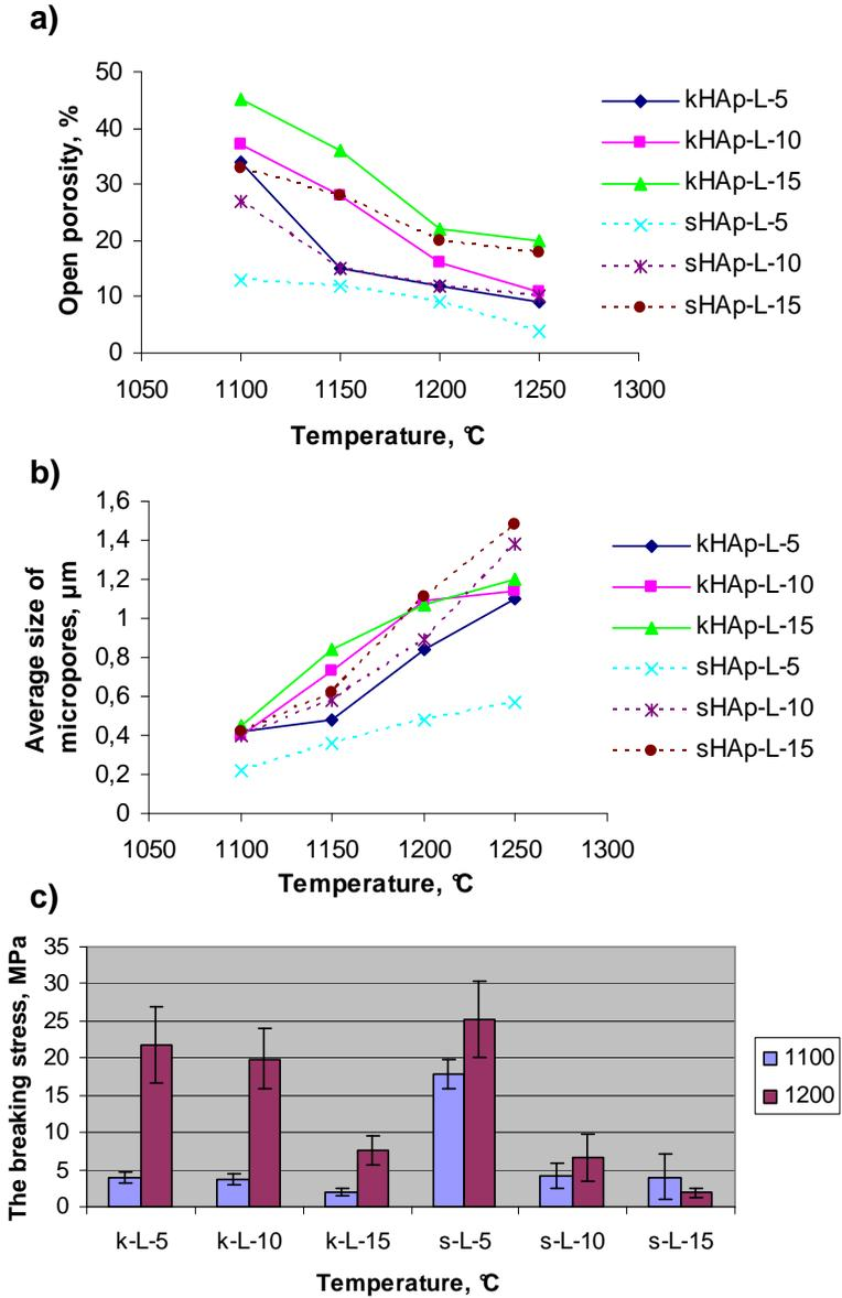
Fig. 6. Open porosity of porous ceramic obtained with lycopodium(a), average size of micropores (b) and the breaking stress at four point bending (c) depending on the sintering temperature.
