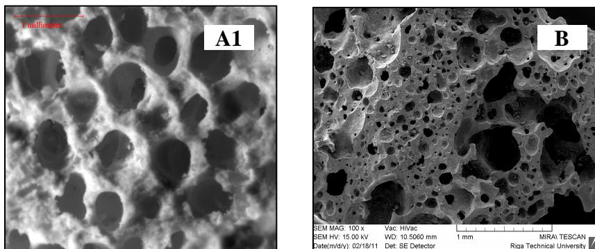
*Fig. 2. Microstructure of porous ceramic precursor polymer (A1) and the ceramic cast in forms (B)*
