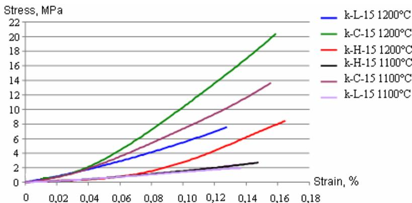
Fig.7. Standard quasi-linear stress-strain curves of samples of uniaxially pressed porous ceramic (pore forming additives L- lycopodium, C- starch, H- chitin)
