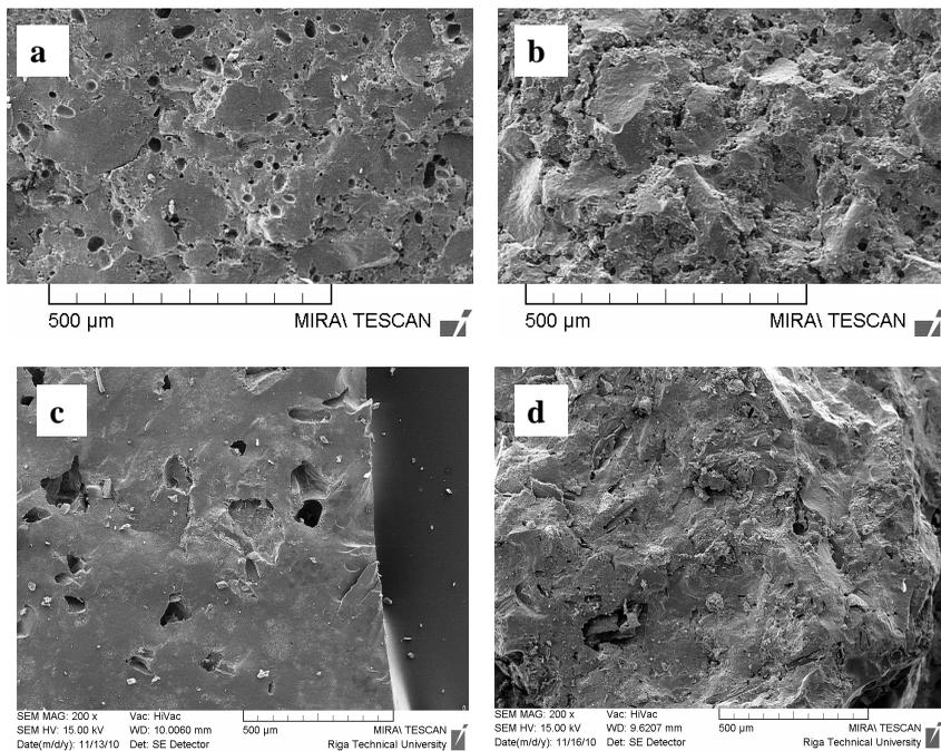
*Fig.3. Microstructure of porous ceramic, with a) starch, b) lycopodium, c) gelatine, d) chitin as pore formers*
