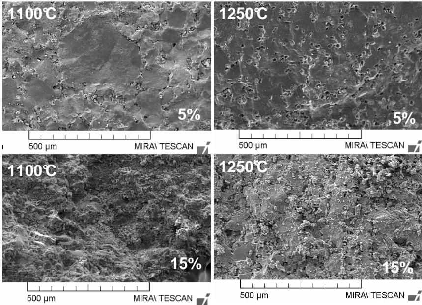
Fig.4. Microstructure of porous ceramic where lycopodium is used as pore former
