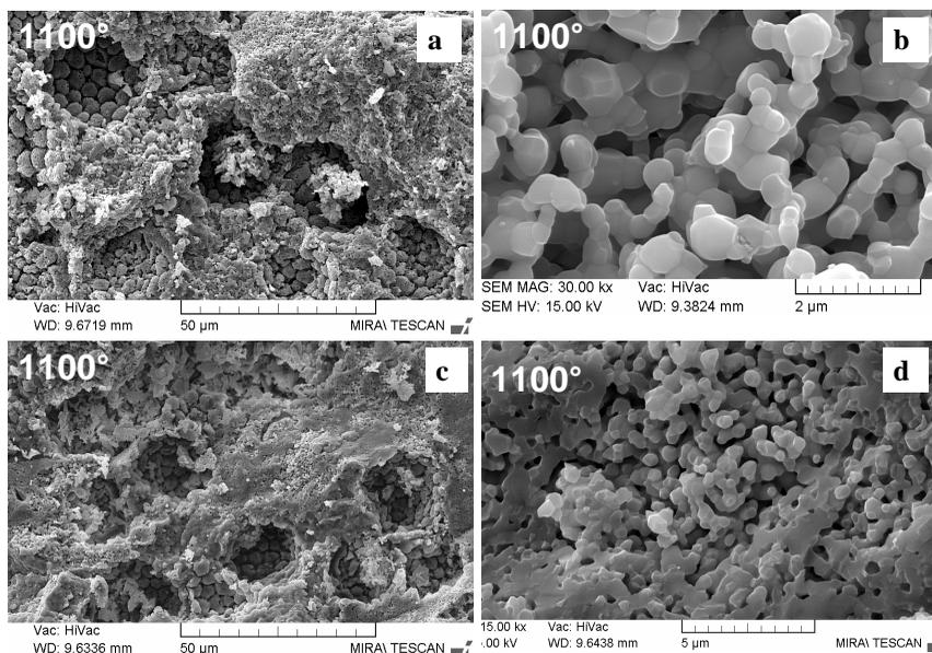
*Fig. 5. Microstructure of porous ceramic on the base of the commercial HAP (a, b) and the synthesized HAP (c, d) with lycopodium as pore former*
