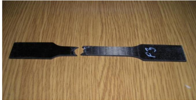
4.fig. Complex reinforced carbon fiber sample after testing
