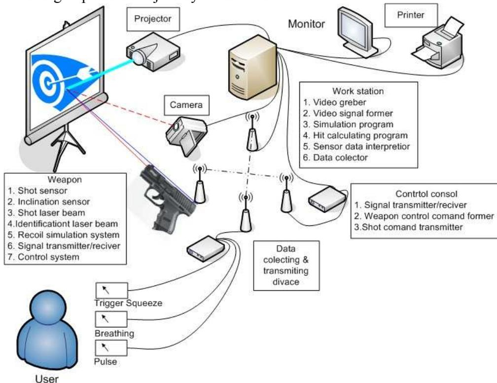
Fig.8. Sensor Integration shooting simulators
