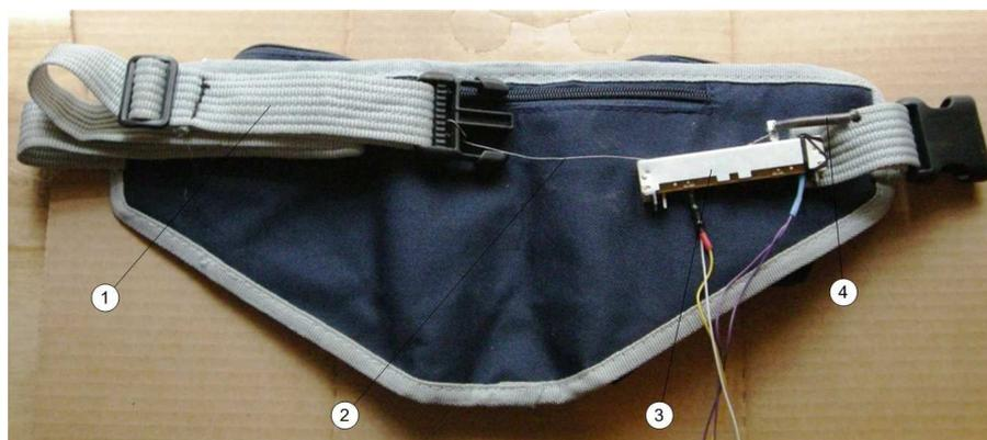
Fig. 12 The breathing sensor acquisition system: 1) Belt, 2) connecting string, 3) the shear stress dividing potentiometer 4) on a slider return spring
