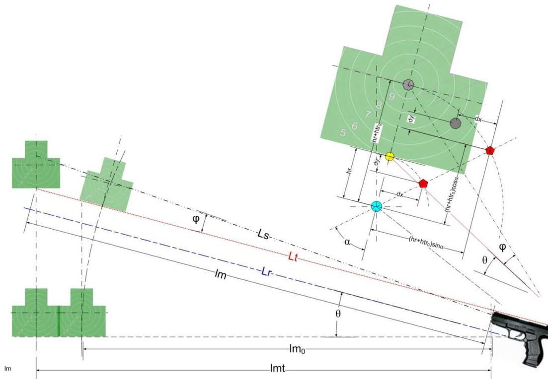
Fig.6. Adjustment of the hit of the gun depends on the elevation angle  $\theta$  to lateral tilt angle  $\alpha$
