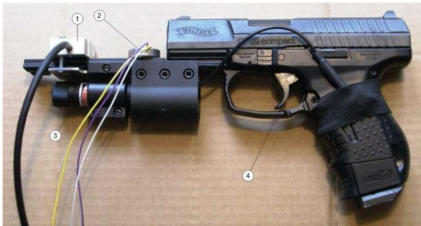
Fig. 11 A gun with sensors: 1) two-way tilt sensor, 2) a microphone, 3) a laser radiant, 4) Walther P99C pneumatic model
