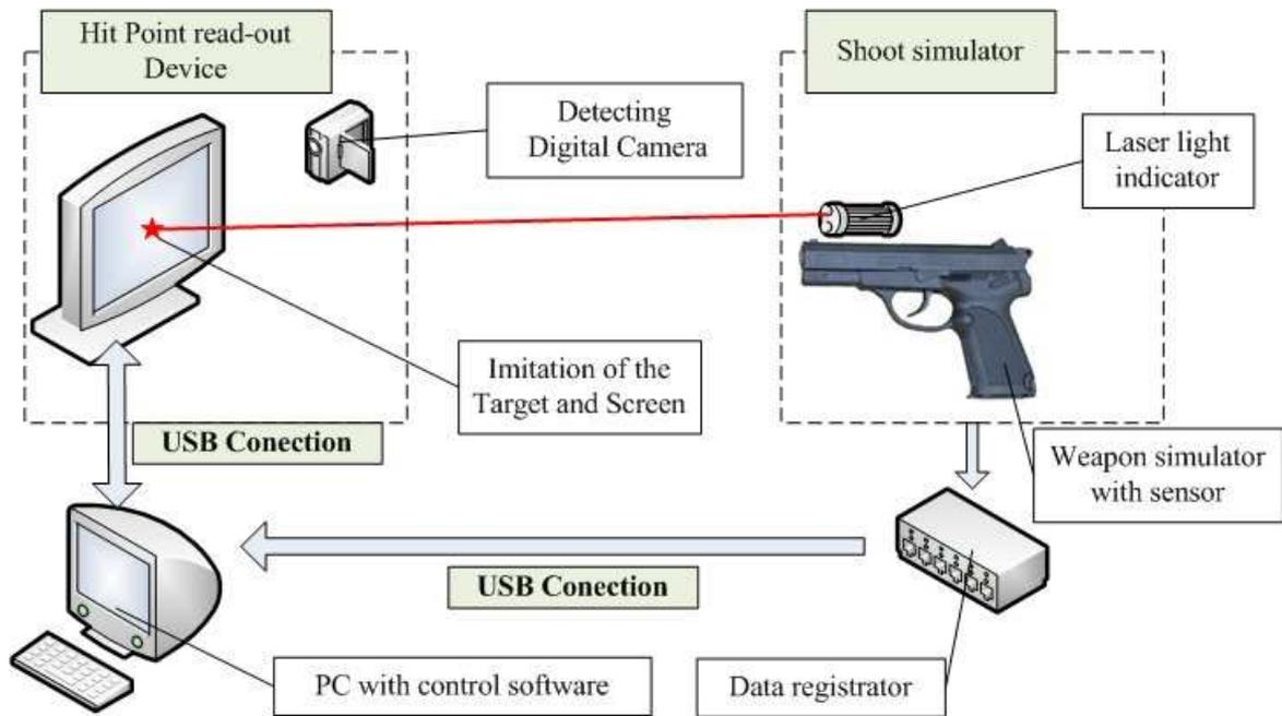
Fig. 9 The shooting simulator block's diagram scheme
