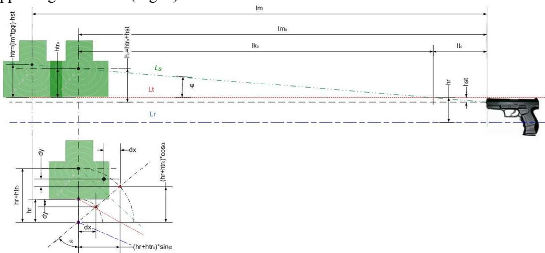
Fig.4. Guns hit the adjustment depending on the side of the tilt angle  $\alpha$
