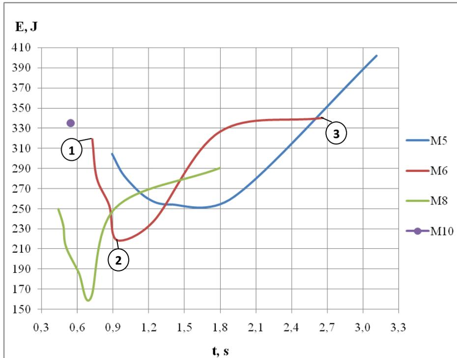
Figure 6.2. The consumption's average values of electric power for corresponding bolts taking into account assembly time
