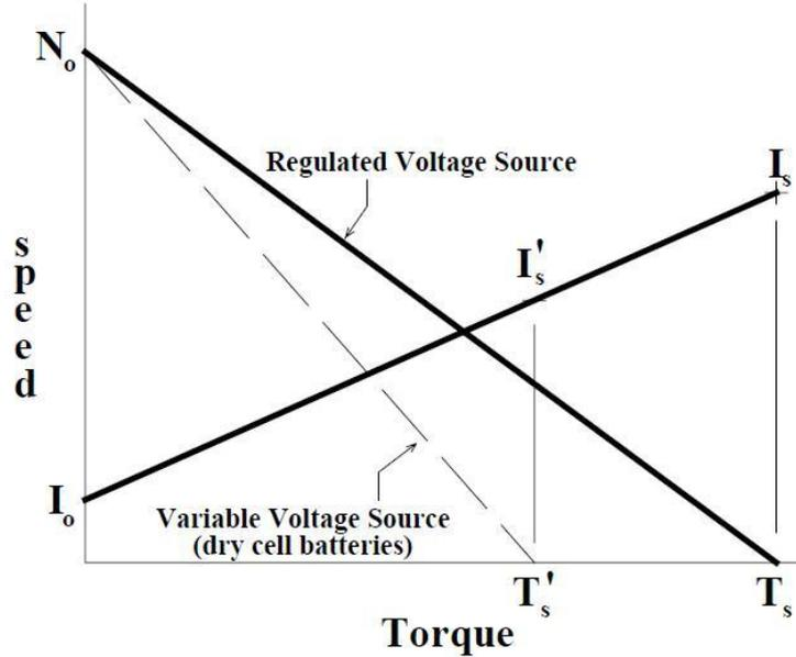
Figure 1.3. Performance Curve Conversion for Battery Voltage Supply
