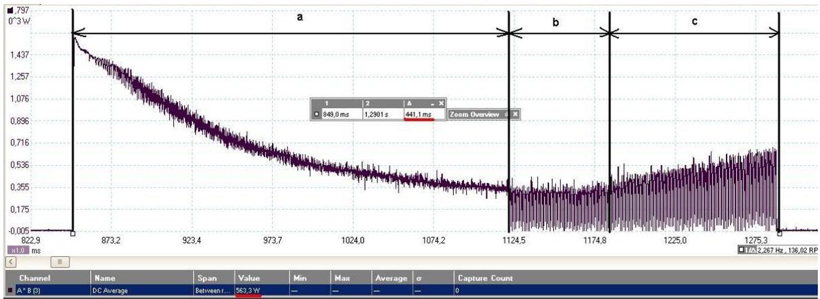
Figure 6.5. 3rd point of the curve. Power consumption for the bolt M6x1,0 by the initial rotation speed  $1500 \text{ min}^{-1}$
