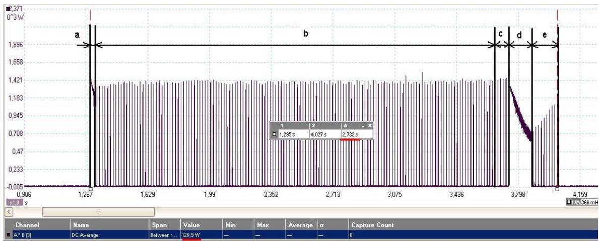
Figure 6.3. 1st point of the curve. Power consumption for the bolt M6x1,0 by the initial rotation speed  $300 \text{ min}^{-1}$
