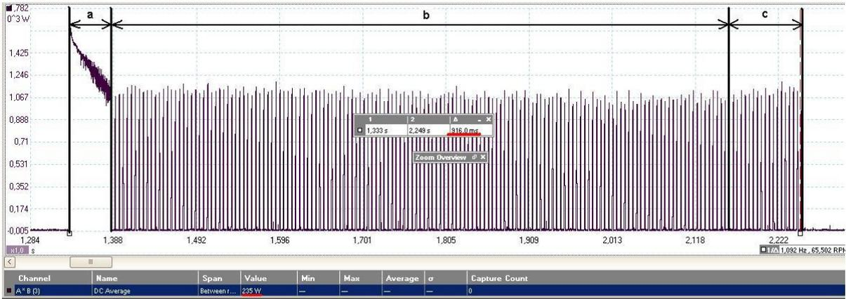
Figure 6.4. 2nd point of the curve. Power consumption for the bolt M6x1,0 by the initial rotation speed  $900 \text{ min}^{-1}$
