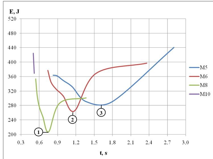
Figure 4.3. Assembly process's theoretically estimated electric power's consumption for the bolts M5, M6, M8 un M10
