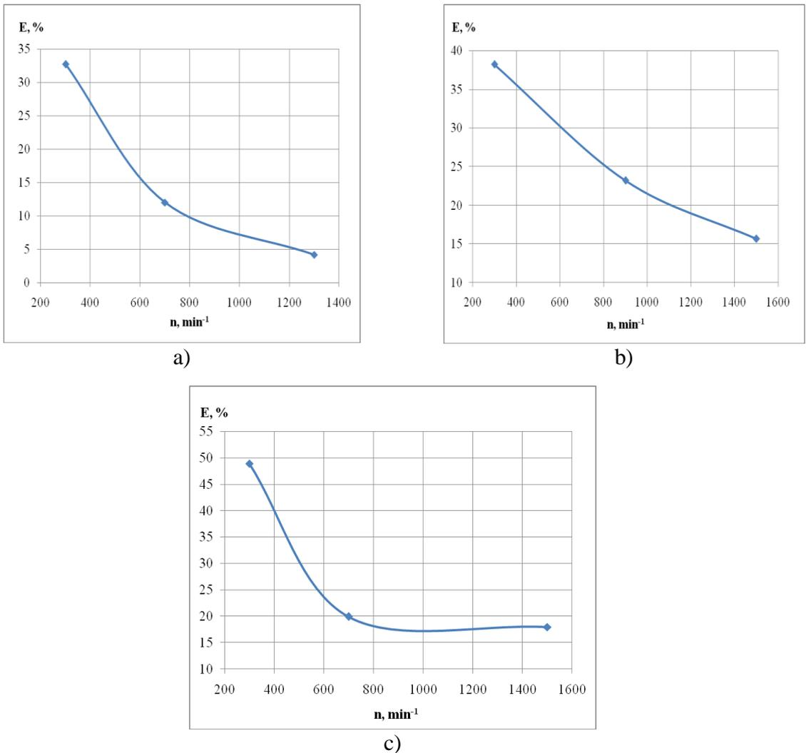
Figure 7.1. The savings of electric power (% from the initial rotation speed)for the bolt: a - M5x0,8; b - M6x1,0; c - M8x1,25
