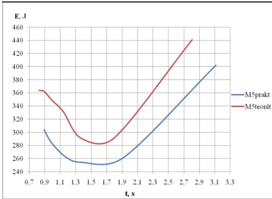
Figure 6.12. Comparison of theoretical and practical values for the bolt M5x0,8
