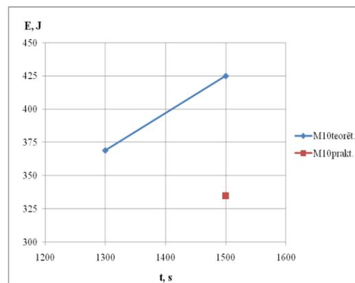
Figure 6.15. Comparison of theoretical and practical values for the bolt M10x1,5
