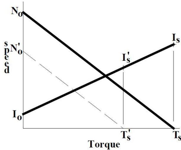
Figure 1.2. Performance Curve Conversion for Different Regulated Voltage Supplies
