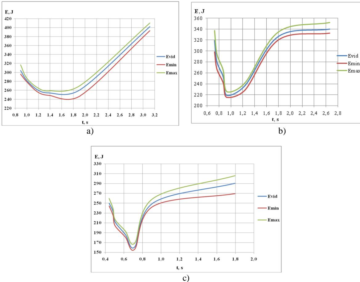
Figure 6.1. The consumption of electric power depending on assembly time for the bolts:
