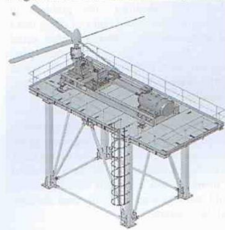
FIGURE 1 SCHEME OF THE TOWER WITH A MODULE INSTALLED FOR WHIRL TOWER TEST
