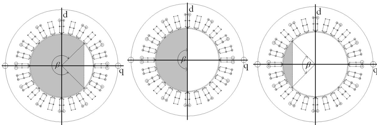
Fig. 2.6.1. SRFC rotor's designs (with gray the ferromagnetic part is shown)
