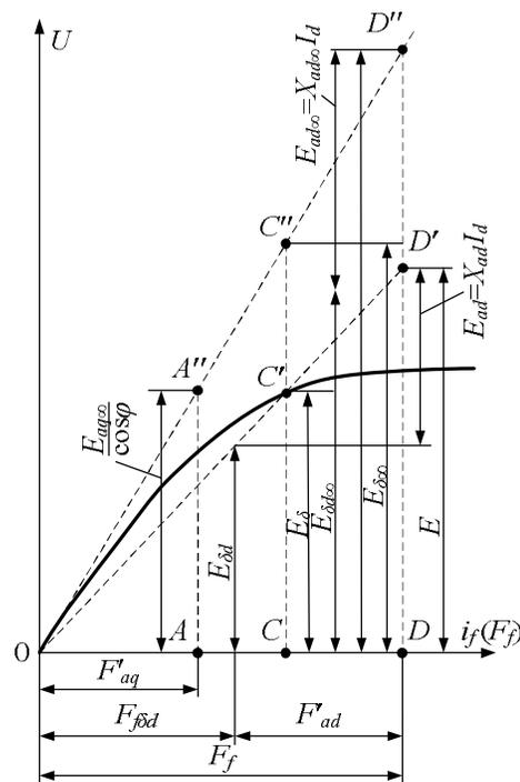
Fig. 2.3.2. Salient pole synchronous generator’s EMF determination (taking into account saturation influence)
