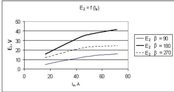
Fig. 2.7.2. In secondary winding induced EMF dependence from armature current if  $\beta = 90^\circ, 180^\circ, 270^\circ$
