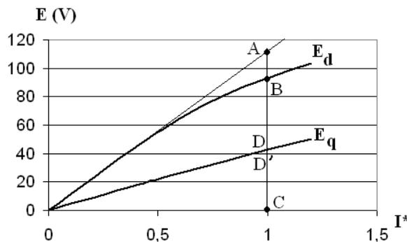
Fig. 2.5.1. Armature winding EMF dependence from armature current (in relative units)
