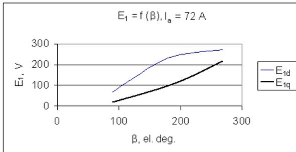
Fig. 2.6.11. In primary winding induced fundamental harmonic EMF effective values dependence from angle  $\beta$ , if  $I_a = 72$  A in direct-axis and quadrature-axis
