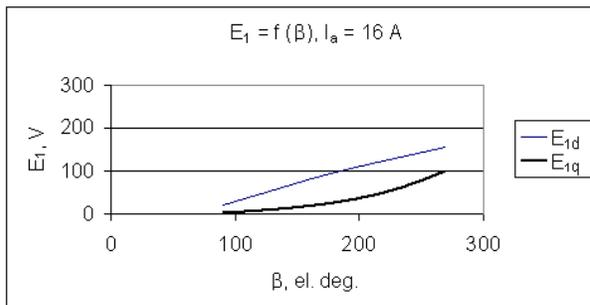
Fig. 2.6.5. In primary winding induced fundamental harmonic EMF effective values dependence from angle  $\beta$ , if  $I_a = 16$  A in direct-axis and quadrature-axis
