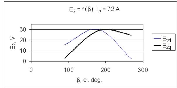
Fig. 2.6.12. In secondary winding induced fundamental harmonic EMF effective values dependence from angle  $\beta$ , if  $I_a = 72$  A in direct-axis and quadrature-axis
