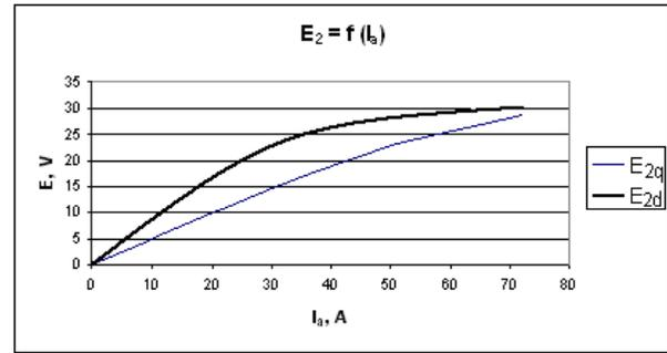
Fig. 2.6.4. In secondary winding induced (direct-axis with index  $d$ , quadrature-axis with index  $q$ ) EMF effective values dependence form armature current for  $\beta = 180^\circ$
