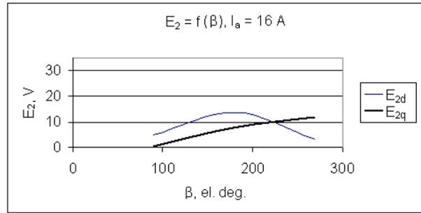
Fig. 2.6.6. In secondary winding induced fundamental harmonic EMF effective values dependence from angle  $\beta$ , if  $I_a = 16$  A in direct-axis and quadrature-axis
