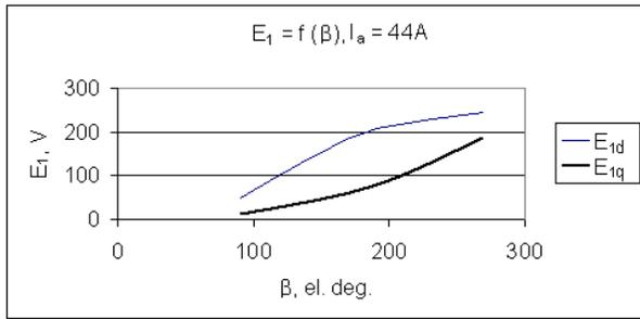
Fig. 2.6.7. In primary winding induced fundamental harmonic EMF effective values dependence from angle  $\beta$ , if  $I_a = 44$  A in direct-axis and quadrature-axis
