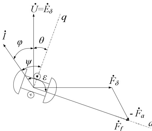
Fig. 2.3.3. Phasor diagram of synchronous machine (engine mode)
