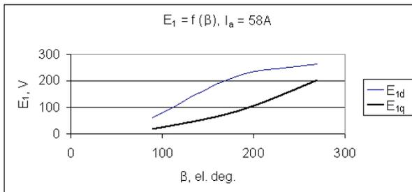
Fig. 2.6.9. In primary winding induced fundamental harmonic EMF effective values dependence from angle  $\beta$ , if  $I_a = 58$  A in direct-axis and quadrature-axis
