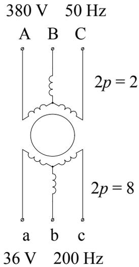
Fig. 2.1.1. Stator winding's scheme
