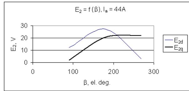
Fig. 2.6.8. In secondary winding induced fundamental harmonic EMF effective values dependence from angle  $\beta$ , if  $I_a = 44$  A in direct-axis and quadrature-axis
