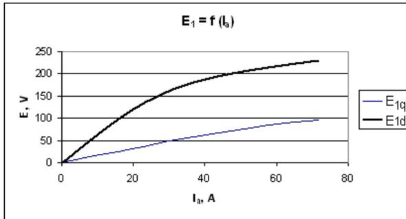
Fig. 2.6.3. In primary winding induced (direct-axis with index  $d$ , quadrature-axis with index  $q$ ) EMF effective values dependence form armature current for  $\beta = 180^\circ$
