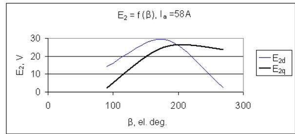
Fig. 2.6.10. In secondary winding induced fundamental harmonic EMF effective values dependence from angle  $\beta$ , if  $I_a = 58$  A in direct-axis and quadrature-axis
