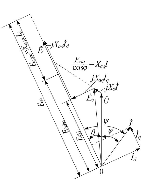
Fig. 2.3.1. Saturated synchronous machines voltage phasor diagram
