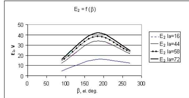
Fig. 2.7.3. In secondary winding induced EMF dependence from rotor's ferromagnetic parts filling angle  $\beta$
