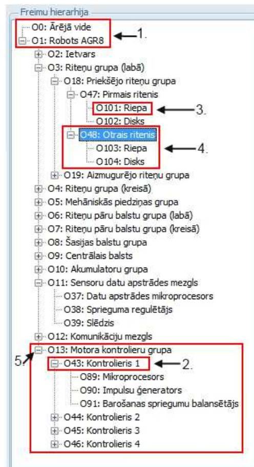
**Fig. 4.1. Frame hierarchy for the system robot AGR8**
