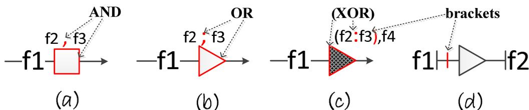
**Fig. 2.3. The representation of logical operators**
