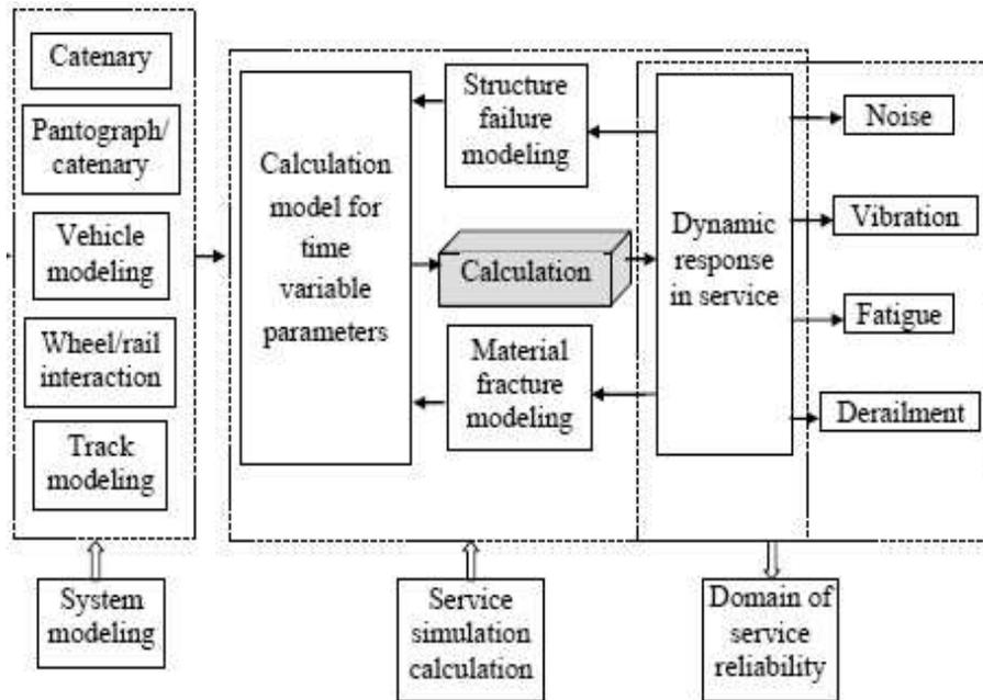
Figure 1. Computer simulation of service reliability for high-speed trains
