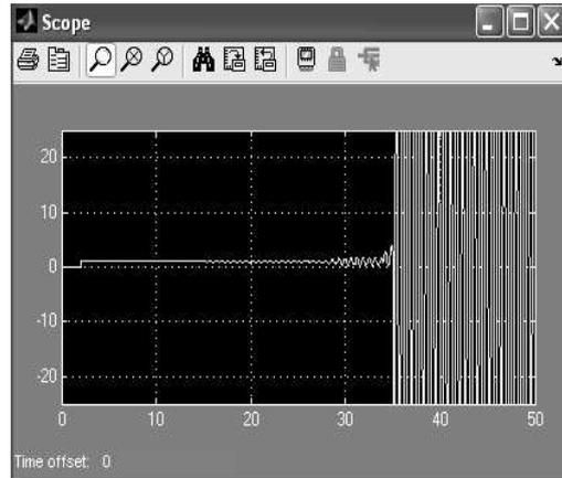
Figure 3b. Transient response of the system with controller with constant parameters
