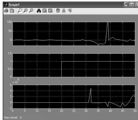
Figure 1b. Transient response of the catenary (upper), transient response of the pantograph (bottom)
