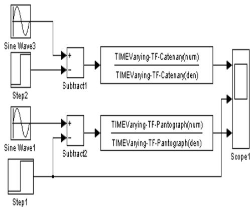
Figure 1a. Schemes of the pantograph and catenary models
