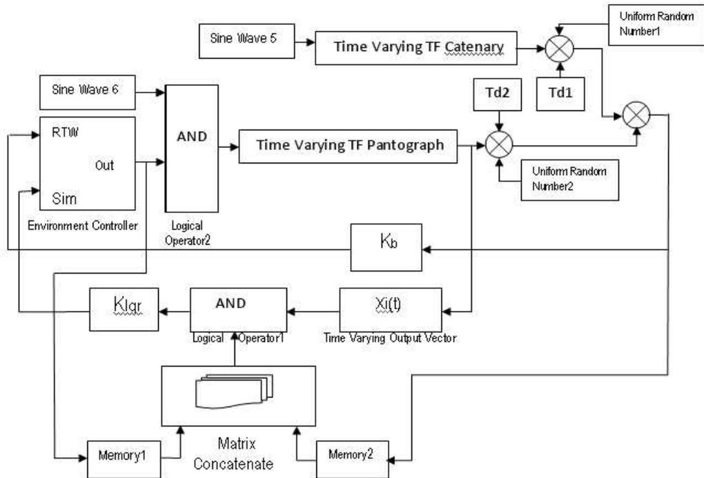
Figure 5. Scheme of the pantograph-catenary model with adaptive controller
