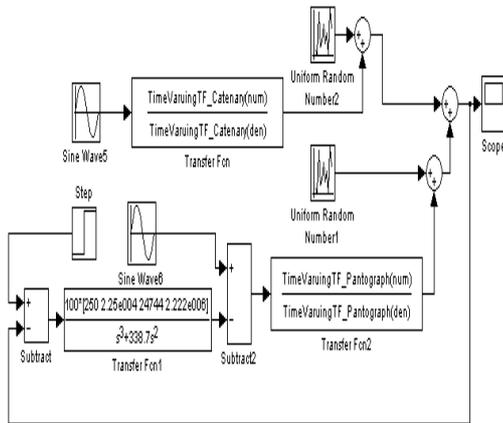
Figure 3a. Scheme of the system with controller (active pantograph)
