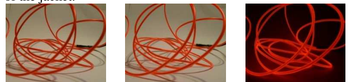
Fig. 11. Comparison of EL wire modes: in the daytime switched off (a) and switched on (b); at night switched on (c)
