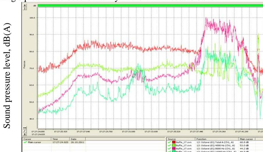
4.17. fig. Electric train braking noise levels in time and frequency domain
