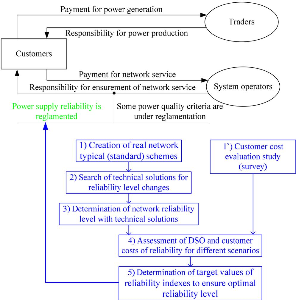
Fig. 6.2. Determination of power supply reliability indexes’ target values as reglamentation of power supply reliability
