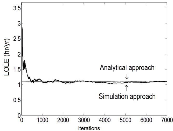
Fig. 5.5. Calculation of LOLE value using analytical and simulation approaches
