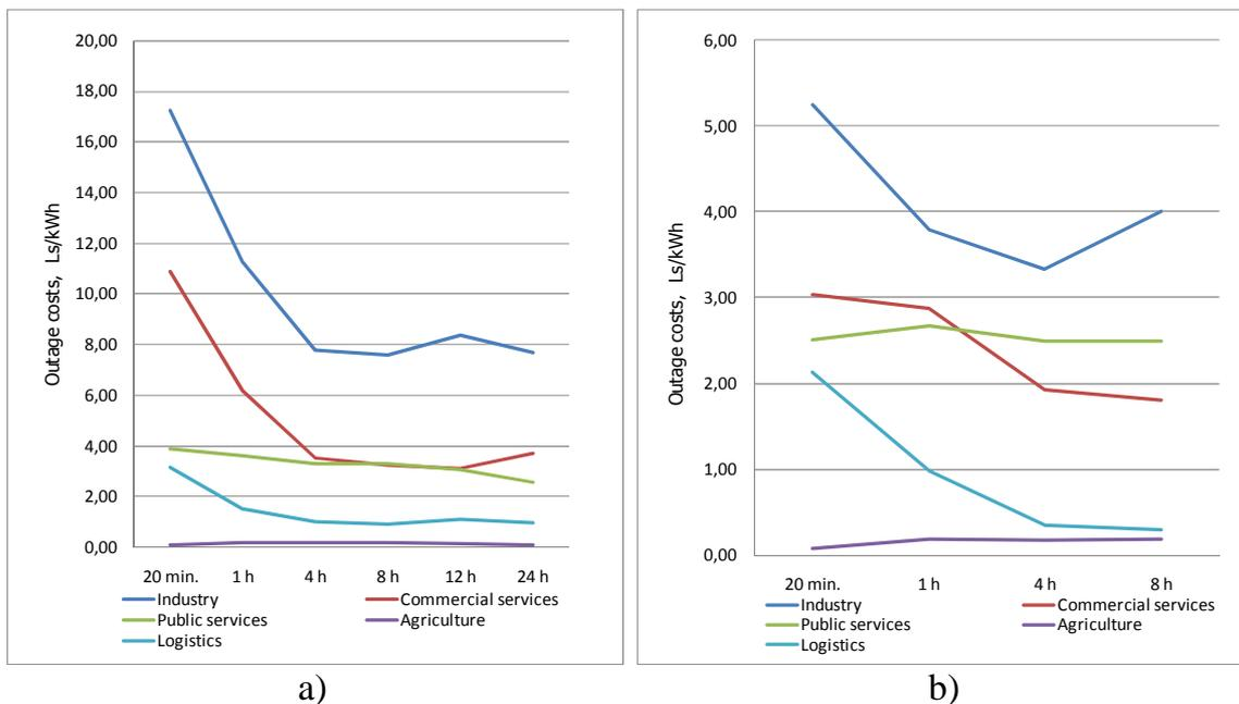
Fig. 4.10. Outage costs, normalized by ENS, caused by: a) unplanned power supply interruptions; and b) planned power supply interruptions
