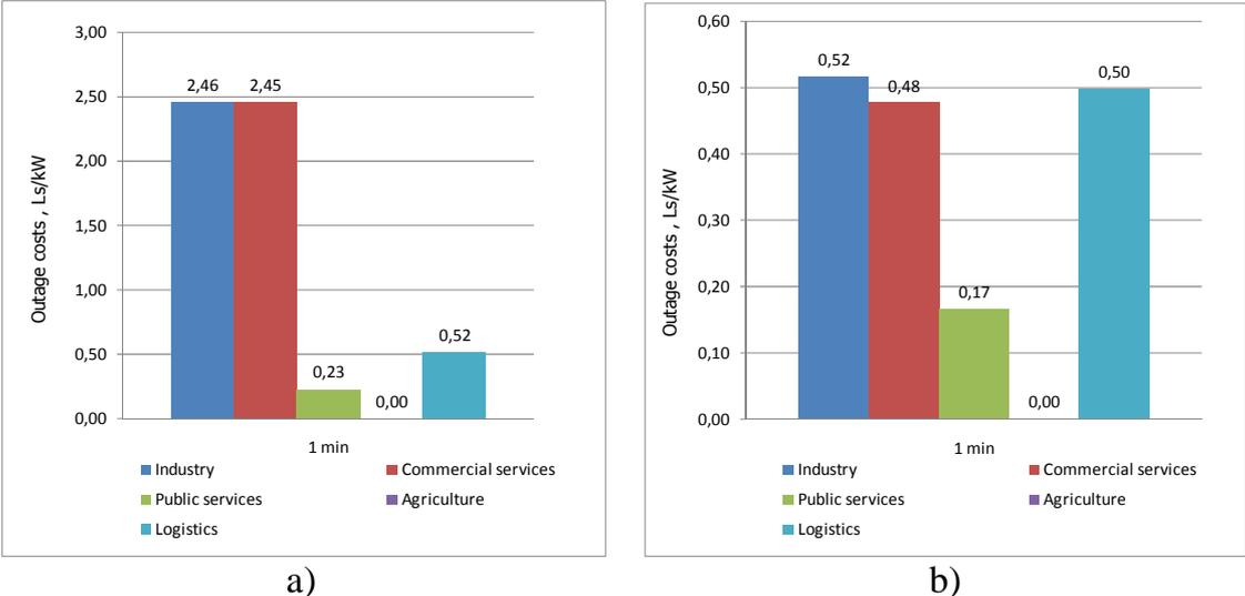
Fig.4.9. Momentary outage costs. Cost values normalized: a) with load interrupted at reference time; b) with maximal allowed power
