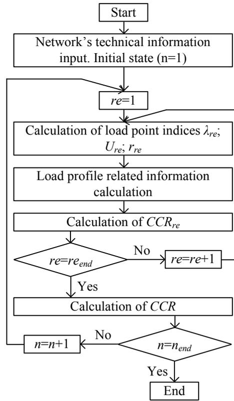
Fig. 5.12. Algorithm for sequence of operations for the process of evaluation of total volume of customer costs of reliability
