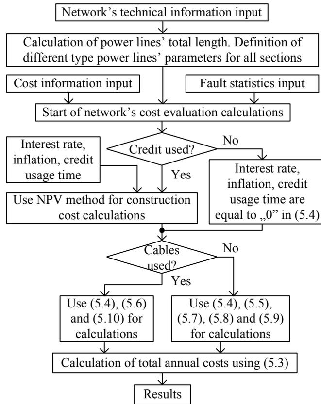
Fig. 5.15. Algorithm for system operator cost assessment
