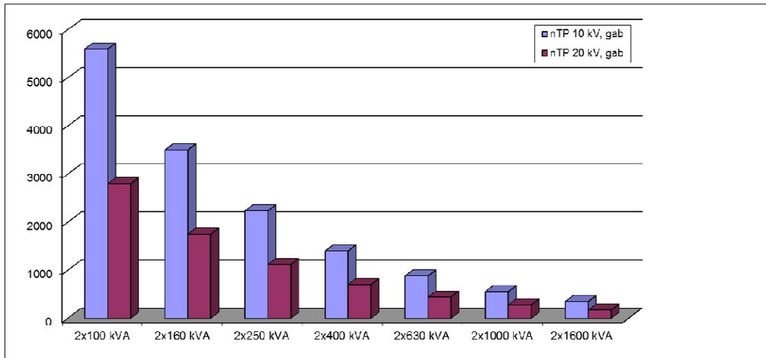
Fig. 4.4. Dependence of the number of 10/0.4 kV and 20/0.4 kV TP in the 110-10-0.4 kV and 110-20-0.4 kV UPSS on the TP power. (at  $\Pi_{city}=74$ km<sup>2</sup>,  $S_{TS} = 2 \times 40$  MVA un  $\sigma_{vid}=9$  MVA/km<sup>2</sup>)
