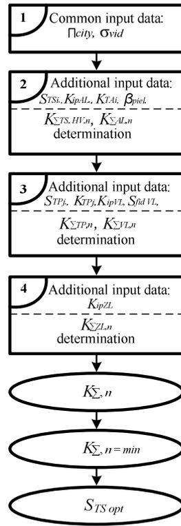
Fig. 3.7. Block diagram for determining of the optimal power of 110/10 kV or 110/20 kV TS
