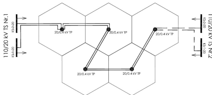
Fig. 3.6. The model of 20 kV network with 20/0.4 kV TP and 20 kV dual-beam cable lines
