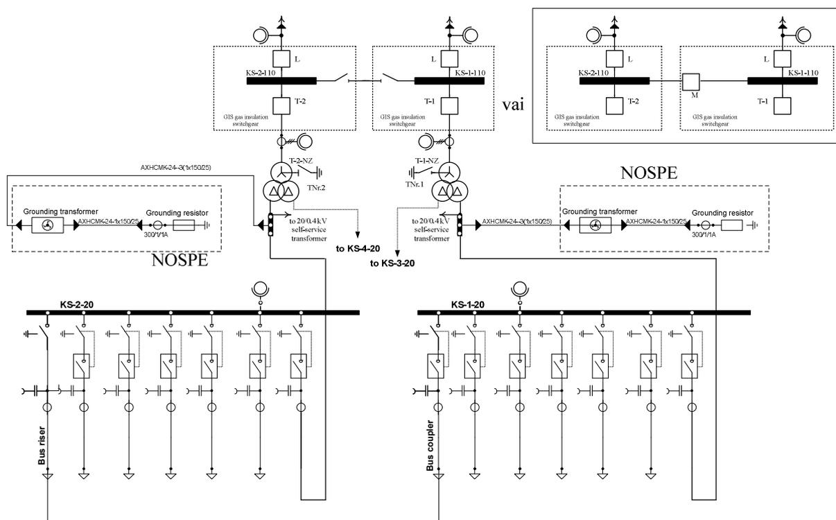
Fig. 5.3. The principal scheme of the proposed 110/20 kV TS
