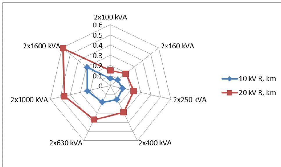
Fig. 4.5. Graph representation of 20/0.4 kV TP and 10/0.4 kV TP service radius of one 2x40 MVA TS at the load density  $\sigma_{vid}=9$  MVA/km<sup>2</sup>
