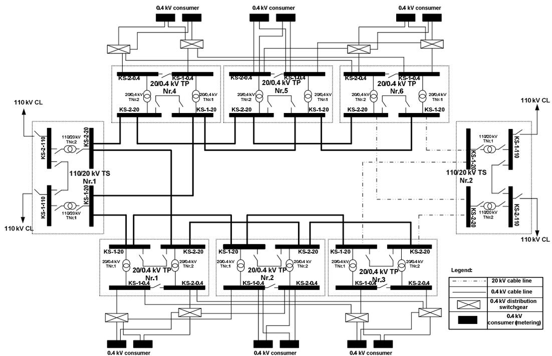
Fig. 5.2. Ideal "dual-beam" power supply scheme of 110-20-0.4 kV UPSS
