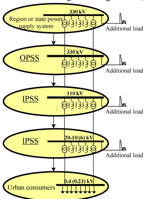
Fig. 1.1. The structure of voltage levels in Latvian power supply system:
