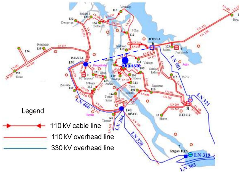
Fig. 1.3. The 330-110 kV network's power supply scheme of Riga city
