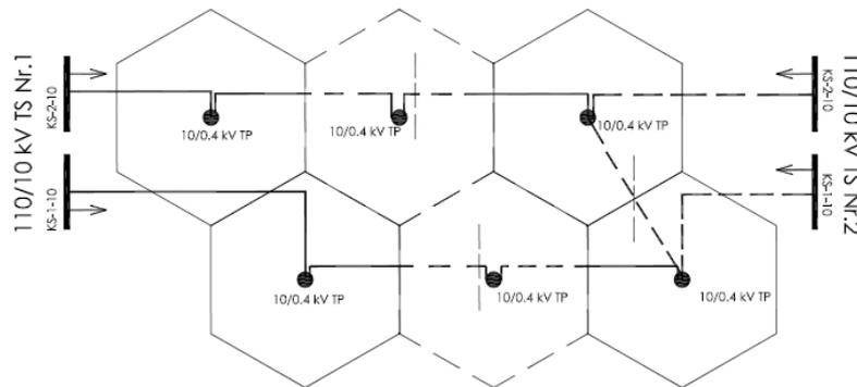
Fig. 3.5. The model of 10 kV network with 10/0.4 kV TP and 10 kV loop-type cable lines
