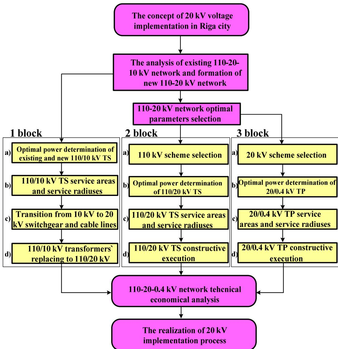
Fig. 3.1. Block diagram of conception of 20 kV voltage introducing in Riga city
