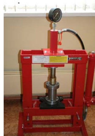
Fig. 2. Experimental setup for pressure application to the specimens.
