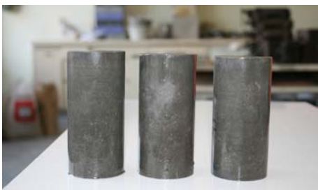
Fig. 3. Looking from the left: the specimens prepared by applying the pressure of 10; 30 and 50 MPa.
