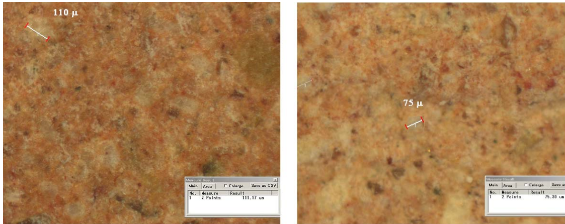
Fig. 1. Dolomite ceramics samples micro cut pictures, taken with microscope "Keyence VHX-300".
