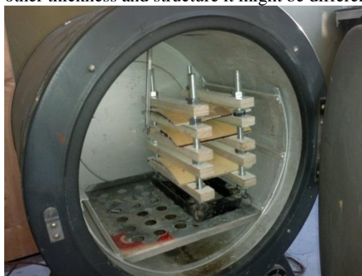
Fig. 11. Thermal box which was used in thermal treatment of samples.
