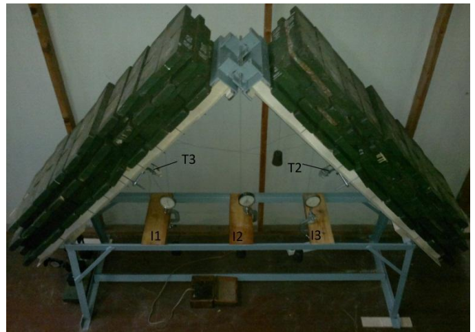
Fig. 18. Experimental roof model, which is loaded with load case No.9. (14 KPa uniformly distributed) by steel weights.
