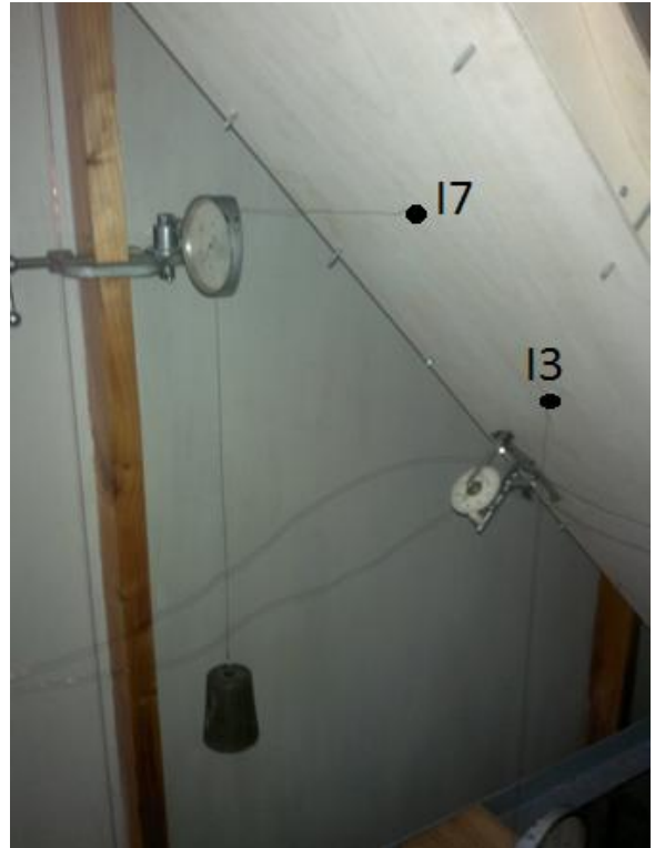
Fig. 17. Outofplane displacement measuring device in point 17 (PAO 102) with precision 0.01mm.
