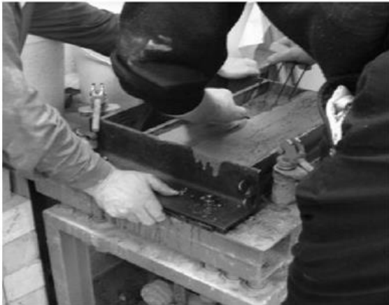
Fig.2. Combing the fibers on the vibrating table
