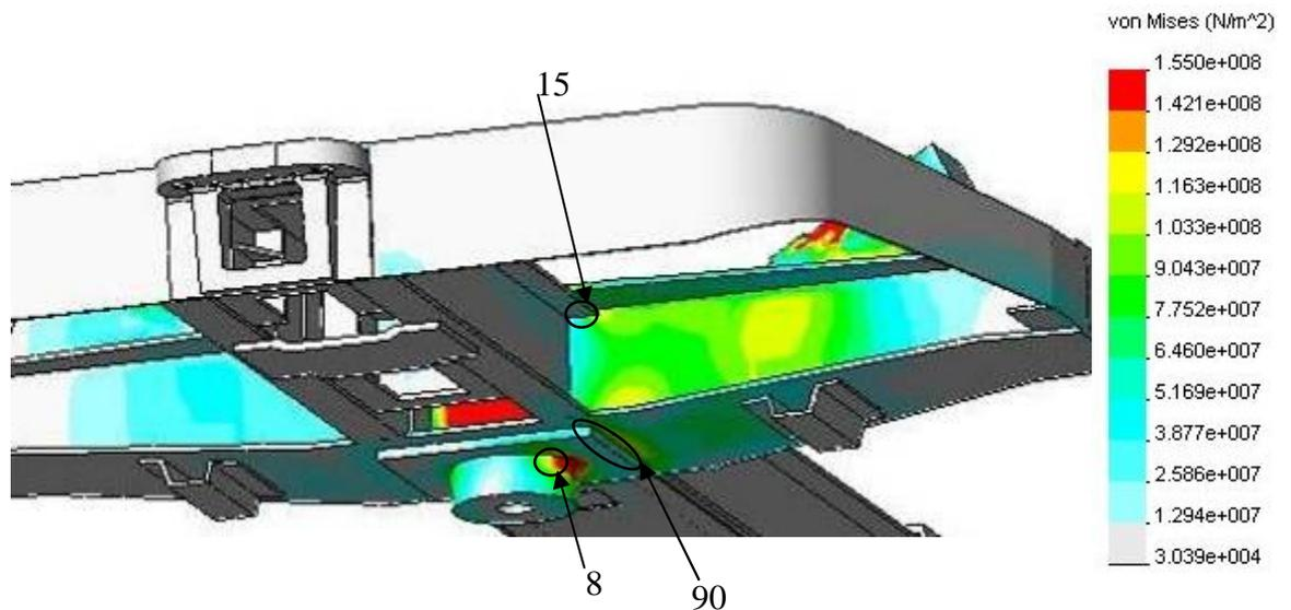
Fig.10b. Distribution of stresses in left support loading, view from bottom
