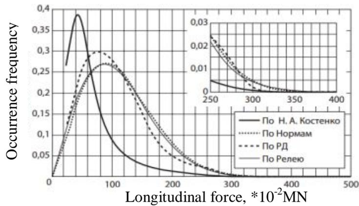
Fig. 2a. Distribution of longitudinal forces by data of Standards [1], what impact freight wagons during operation, comparison with other distribution types and in comparison with Relay distribution
