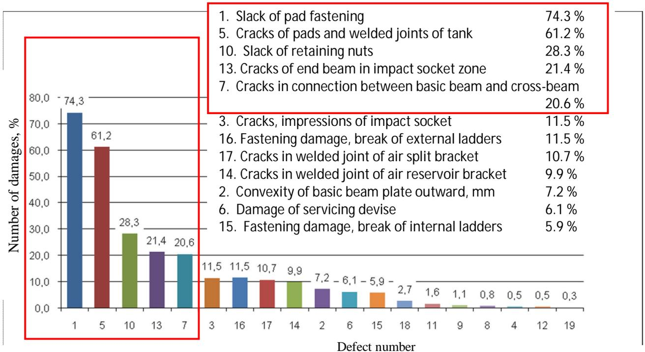
Fig. 3. Distribution of damages towards total number of inspected batch of wagons in amount of 374 tank wagons
