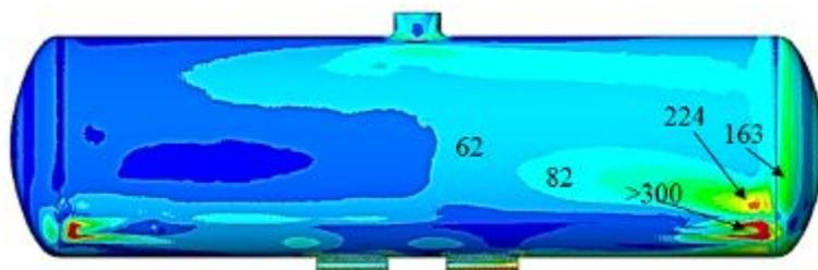
Fig.9. Equivalent stresses in boiler support on upper sill supports, view from side
