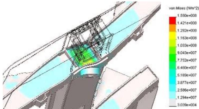
Fig.15. Calculation of lateral swinging regime strength
