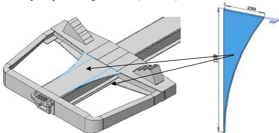
Fig.12. Console part of tank wagon frame
