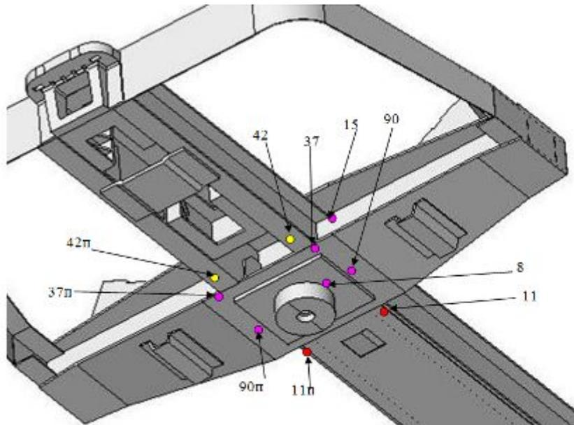
Fig.7b. Location scheme of maximal stress points in distance of 20-25 mm from stress concentrators, view from bottom, turned
