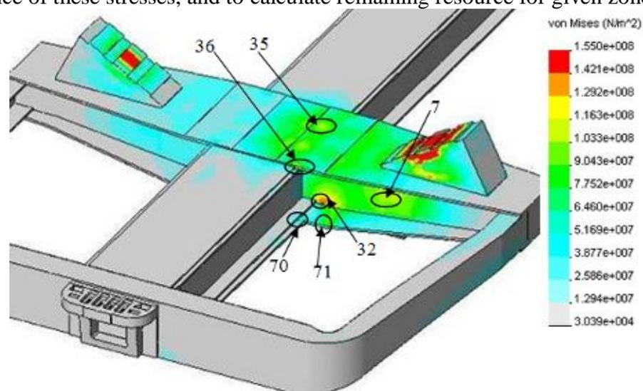
Fig.10a. Distribution of stresses in left support loading, view from top
