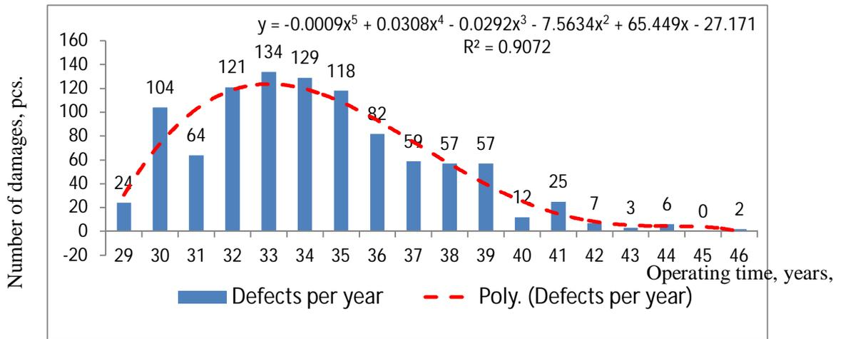
Fig.4. Distribution of damages in tank wagon sample depending on operating time
