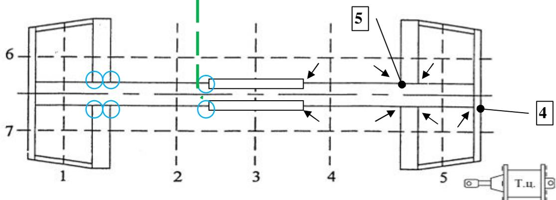
Fig.14.b. Map of inspection zones for frame thickness measurements and damages
