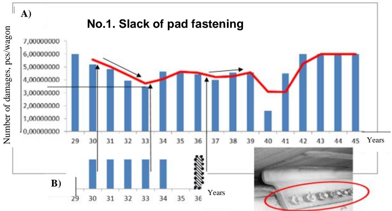
Fig.5. A) Total amount of slacks of pad fastening defects; B) Performance scheme of depot repairs in operational years of tank wagon 30, 31, 32, 33, 34, and performance scheme of capital repairs in year 36
