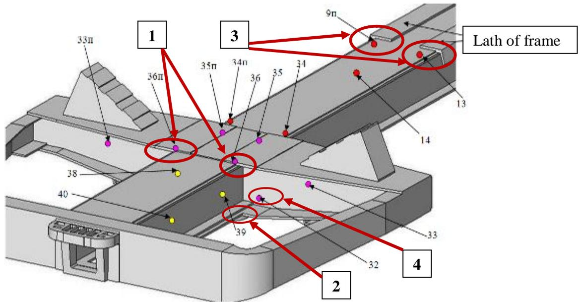
Fig.7a. Location of calculation points of frame, view from top, turned
