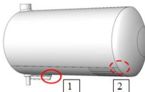
Fig.6. Calculation model of ¼ boiler: 1- welded joints of pads, 2 – connection of T-type joints
