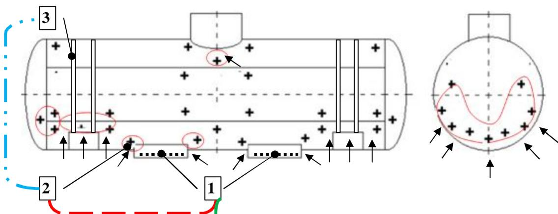
Fig.14.a. Map of inspection zones for boiler thickness measurements and damages
