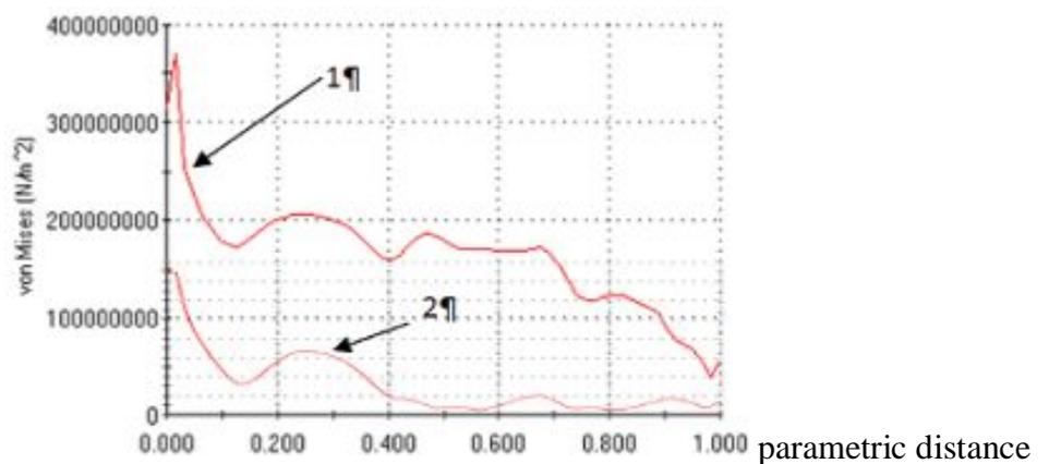
Fig.13. Comparison of frame stresses (strengthening plates in concave external edge) before and after strengthening. 1 – stresses of frame before strengthening, 2 - stresses of frame after strengthening.
