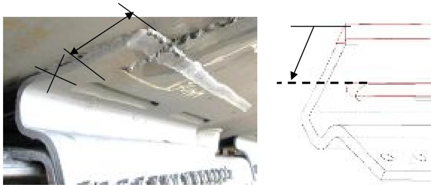
Fig.8. Crack in perpendicular joint of tank wagon pad and model
