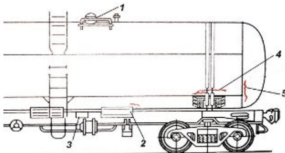
Fig. 1. Zones of tank wagon boiler damages: 1. – welded joints of hatchway; 2 – welded joints of pads; 3 – welded joints of discharging device; 4 – welded joints of boiler edge ring at sill supports; 5 – welded joints of bottom.
