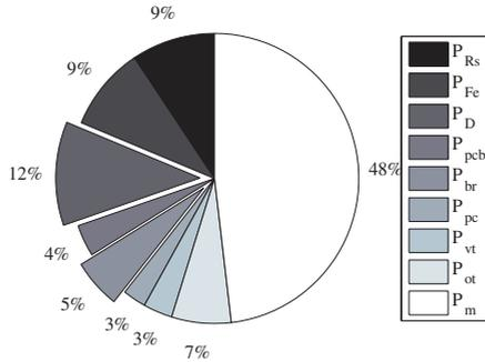
Figure 3.2: Power distribution during a reference application,  $\overline{P}_{ac} = 2293W$
