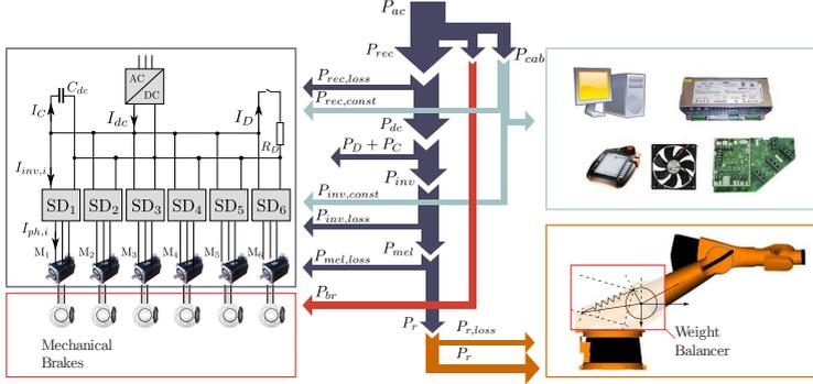
Figure 2.1: Block diagram of a drive system and power components
