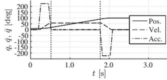
(b) Kinematic profile,  $1/2\dot{q}_{i,max}$ ,  $1/2\ddot{q}_{i,max}$
