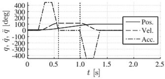
(a) Kinematic profile,  $\dot{q}_{i,max}$ ,  $\ddot{q}_{i,max}$
