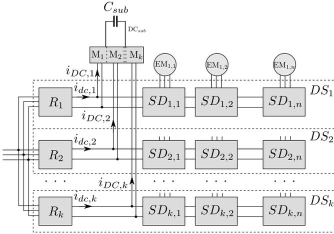
Figure 5.1: Block schematic of a DC subgrid for energy exchange
