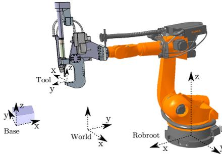
Figure 1.2: 6DOF industrial robot manipulator with a welding tool, overview of coordinate systems.
