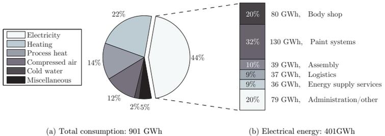
Figure 1.1: Energy consumption in Daimler AG Plant Sindelfingen. Data broken down by type of energy (a); by production centers (b). [21]
