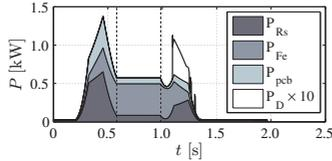
(c) Power losses in robot controller,  $\dot{q}_{i,max}$ ,  $\ddot{q}_{i,max}$
