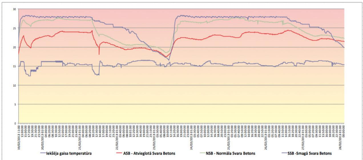
Fig. 2.2. Surface temperature data for various type of blocks
