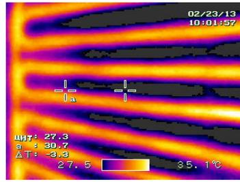
Fig. 2.7: Thermograph of experimental heater
