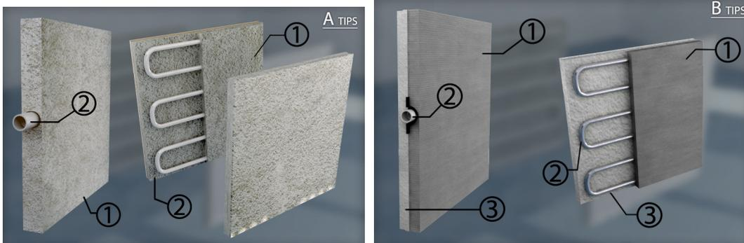
Fig. 1.1 A-type system: pipes built into the dispersing paving or concrete
