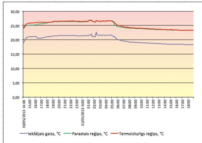
Fig. 2.3. Surface temperature data for different types of drywall
