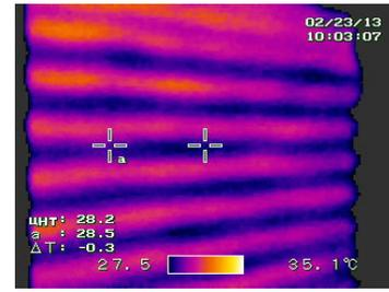
Fig. 2.8: Thermograph of experimental heater
