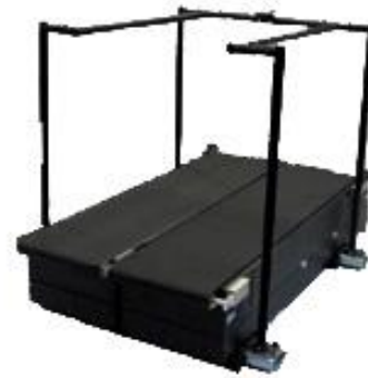
Figure 1.11. Example of instrumented treadmill for GRF measurements [36]
