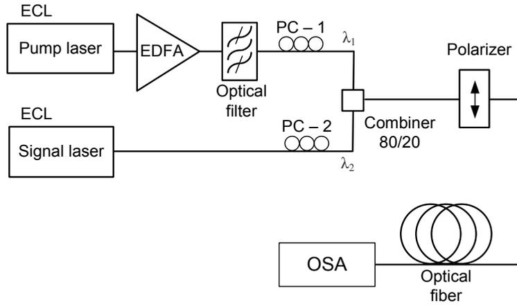
Fig. 8. Experimental  $\gamma$  measurement scheme, using FWM.
