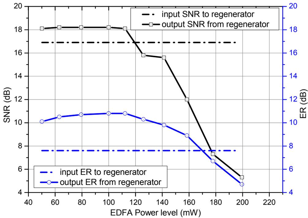
Fig. 14. Input and output optical signal ER and SNR in fixed filter case at filter shift  $\Delta\lambda=0.7$  nm.
