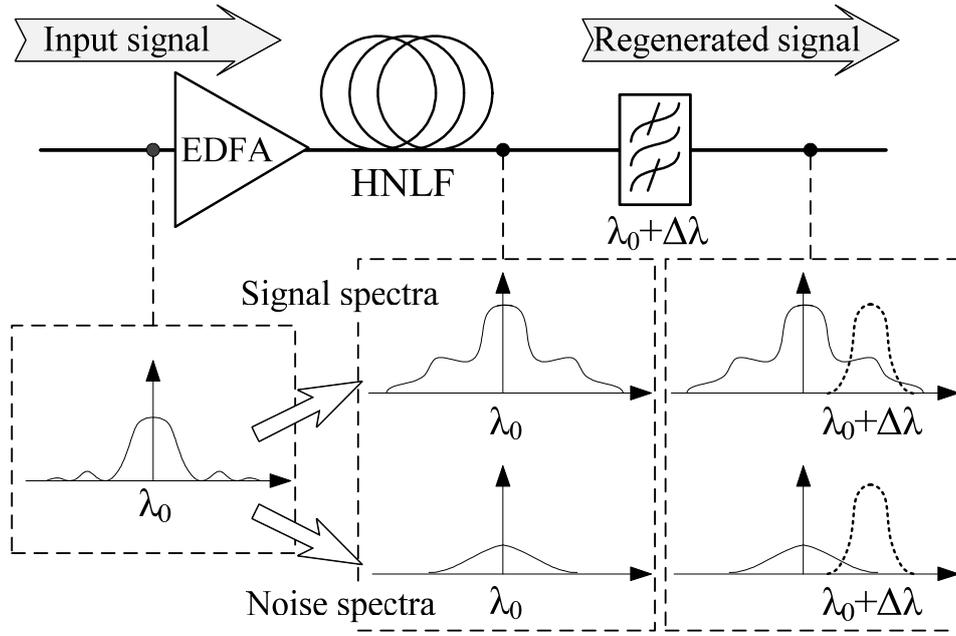
Fig. 11. The operating principle of the Mamyshev type regenerator
