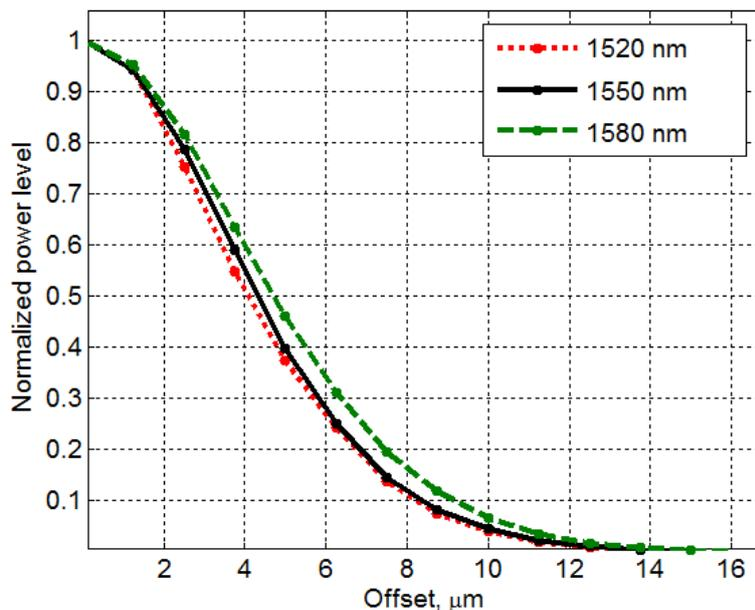
Fig. 5. Normalized optical radiation near-field distribution in fiber cross-section at wavelengths of 1520, 1550, and 1580 nm, depending on the mutual shift of fiber ends.
