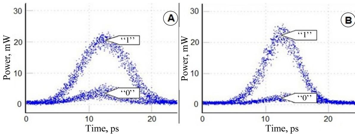
*Fig. 16*. Distorted optical signal in regenerator input (A) and regenerated signal in the output (B) using the tunable filter.
