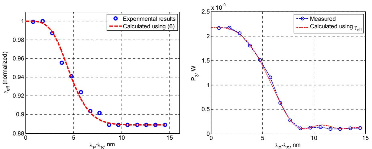
Fig. 10. a) Normalized  $\gamma_{eff}$  depending on  $\Delta\lambda$  between the pumped and signal component.
