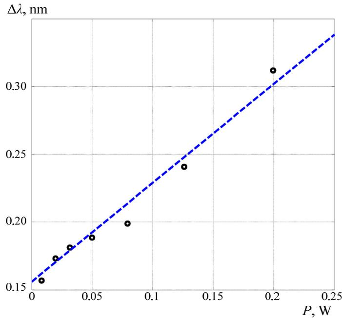
Fig. 7. Measurement results obtained with the P-SPM method and their linear approximation (the blue dotted line) for G.652 D type fiber.
