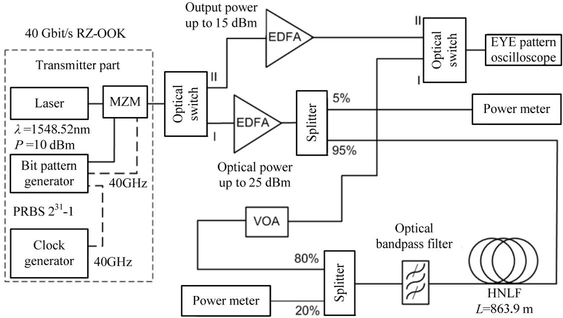
Fig. 12. Scheme of the developed experimental regenerator.
