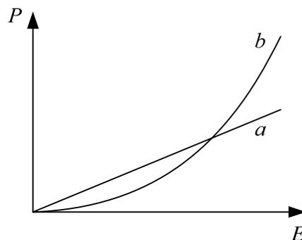
*Fig. 2.* Correlation between  $P$  and  $E$  in case of linear (a) and nonlinear (b) dielectric medium [9].
