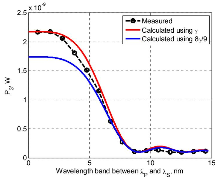
Fig. 9. Calculated and measured FWM component ( $\lambda_{FWM} = 2\lambda_p - \lambda_s$ ) power depending on the pump ( $\lambda_p$ ) and signal ( $\lambda_s$ ) component wavelength difference.
