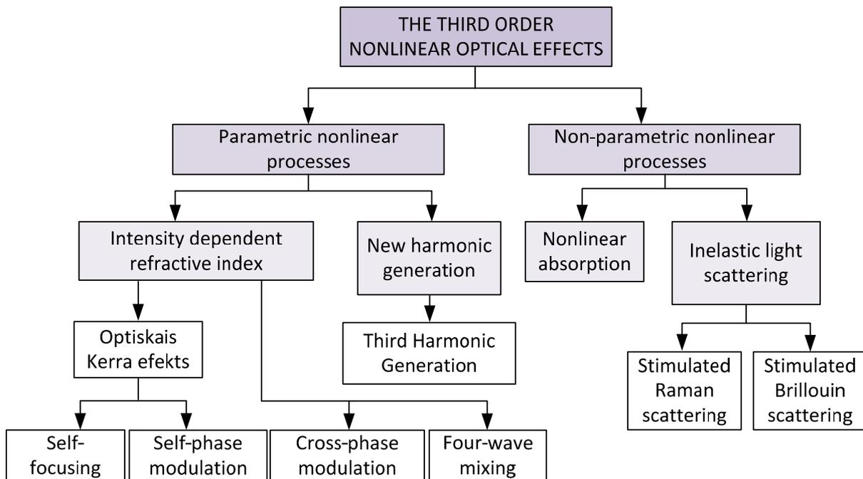
Fig. 3. Classification of third order NOE observed in optical fibers.
