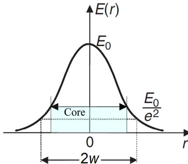
Fig. 4. Optical radiation in a single mode optical fiber with the Gaussian distribution. The mode field diameter is the function width  $2w$  at level  $1/e^2$  [15]. The light blue denotes the fiber core diameter.
