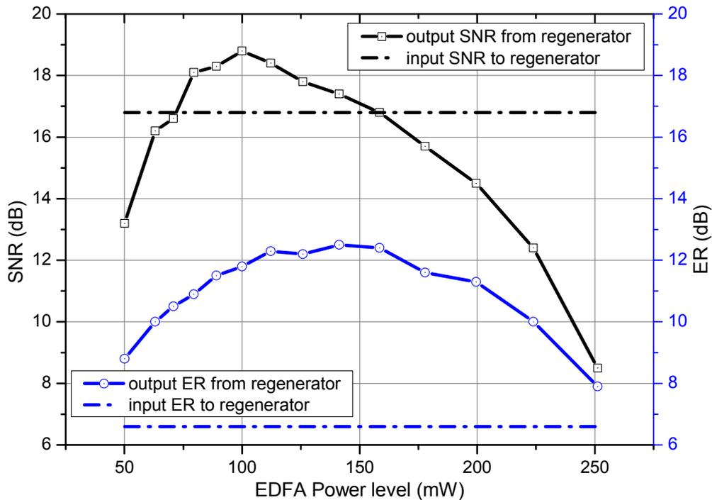
Fig. 15. Input and output optical signal ER and SNR in tunable filter case at filter shift  $\Delta\lambda=0.7$  nm.
