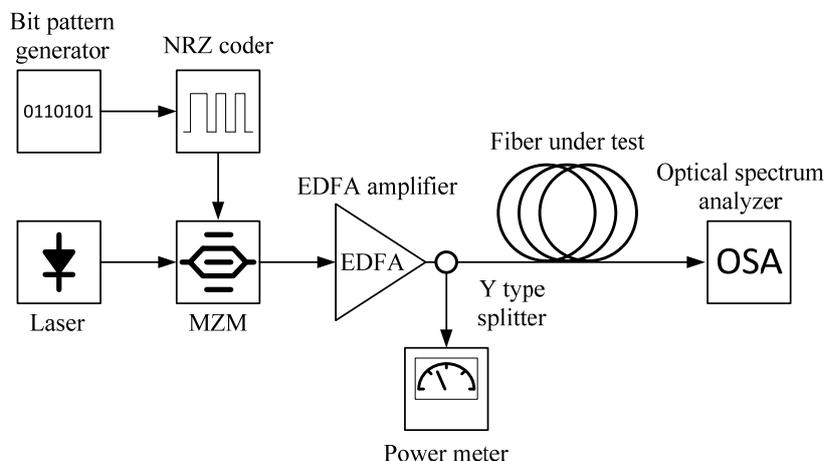
Fig. 6. Simulation and experimental P-SPM nonlinear coefficient measurement scheme based on the use of SPM nonlinear effect.
