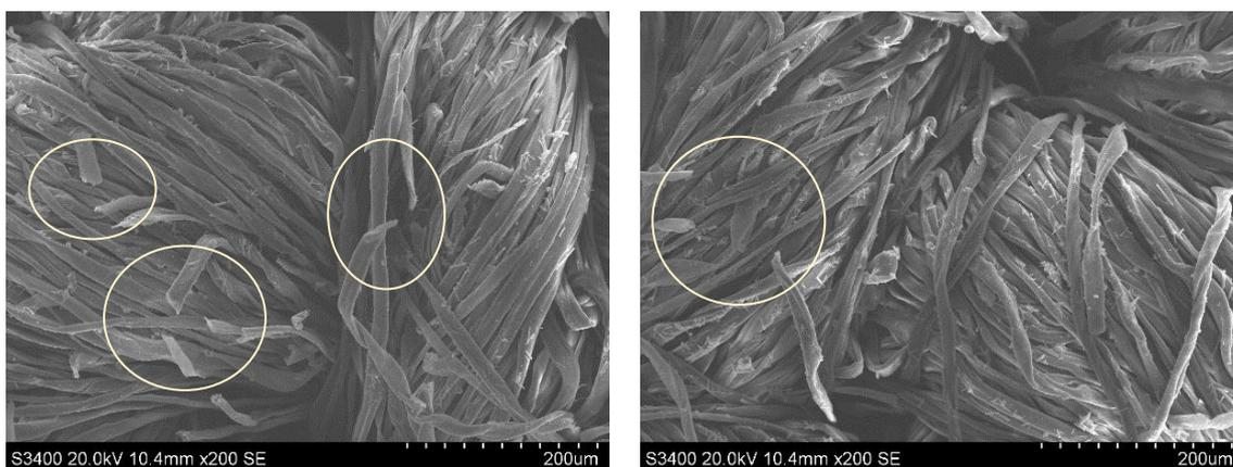
Fig. 5 The cotton textile modified by 5 wt. % ZSH (0.1 M TEOS) sol (thermal post-treatment at 120 °C temperature 2 min.)
