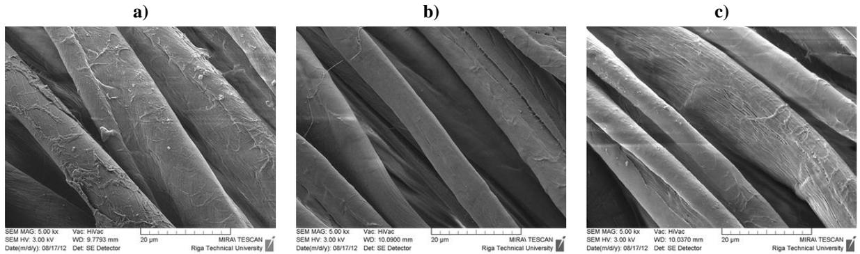
Fig. 2 Influence of the plasma treatment on cotton textile fibre
