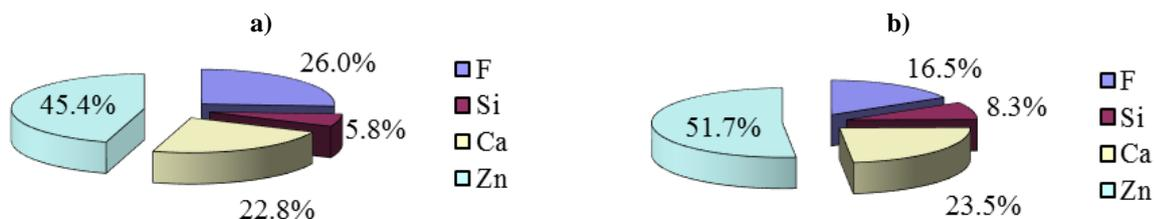
Fig. 8 Relative percentage weight of the chemical elements on the surface of textile treated by 7.5 wt.% ZAD (0.1 M TEOS) sols, after 50 cycles of hydrothermal treatment
