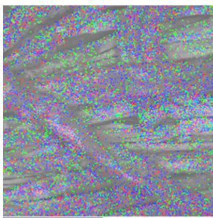
20. Fig. The distribution of the chemical elements **F**, **Si**, **Zn** in the coating of the modified cotton textile surface
