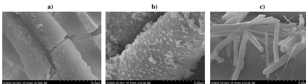
Fig. 4 The coating structure changes depending on the composition of the sol, thermal post-treatment 120 °C at temperature 2 min:
