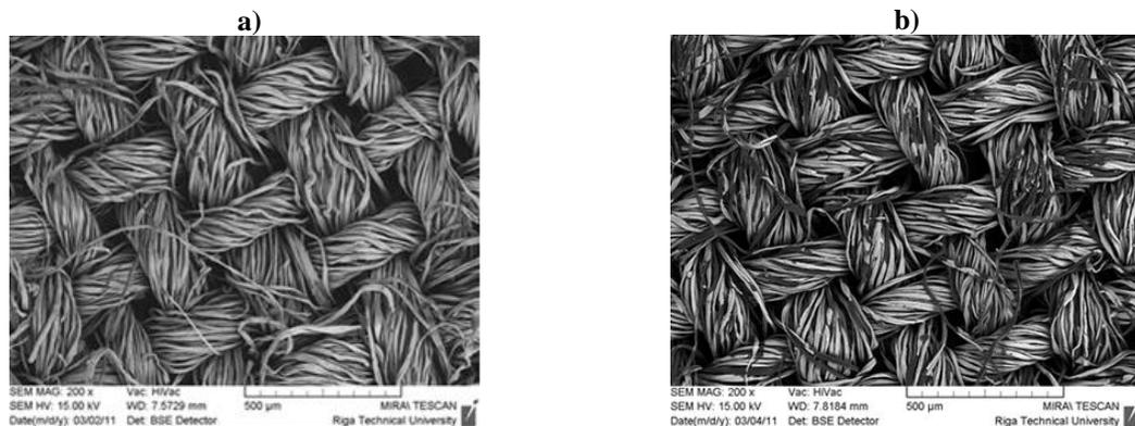
Fig. 3 The copper coating structure on the cotton textile surface deposited by magnetron sputtering technology, coating thickness 90 nm, deposition time 60 s (one sample exposition time 4.5 s):
