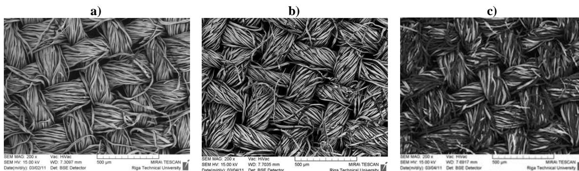
Fig. 1 The copper coating structure on the cotton textile surface deposited by thermal vacuum evaporation technology, copper coating thickness 60 nm (deposition time 1 s): a) coated, b) after one cycle of hydrothermal treatment, c) after one cycle of the hydrothermal treatment: with plasma treatment 3 min before deposition
