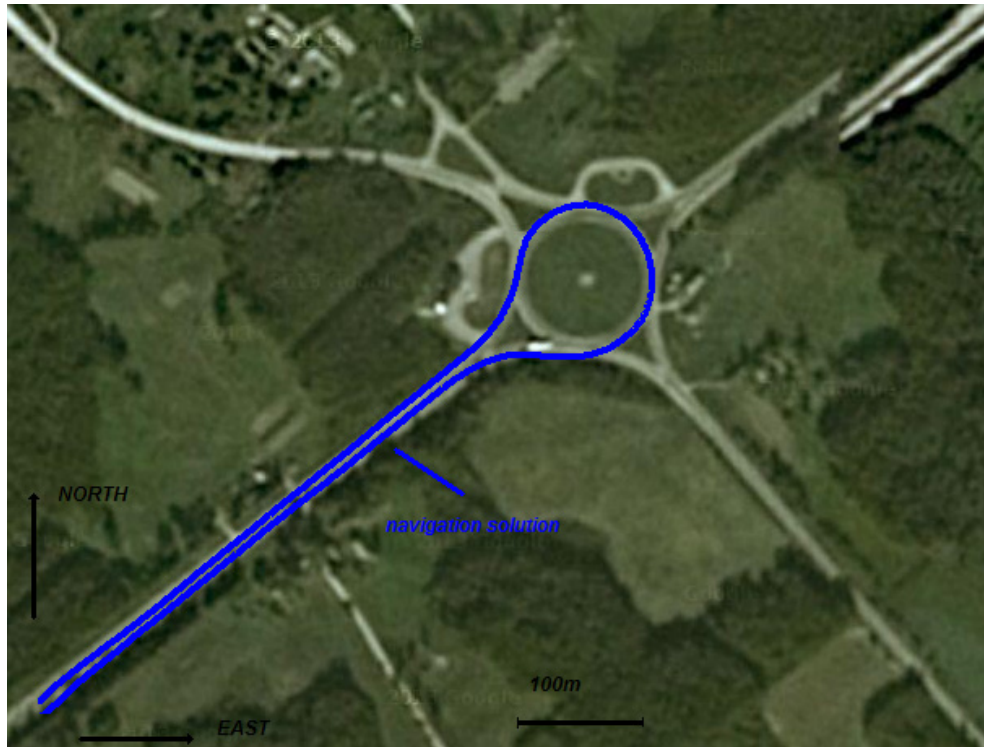
Fig. 5.8. Trajectory estimation of the moving land vehicle (blue curve). TEST Jan2
