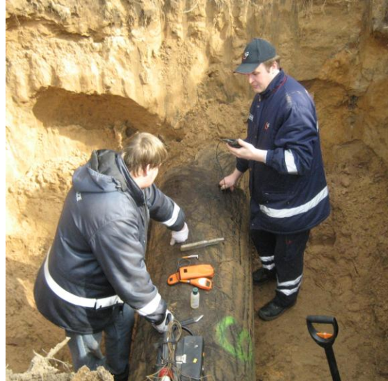
Fig. 1.5 Measuring of the thickness of the wall of a metal pipe in a test pit
