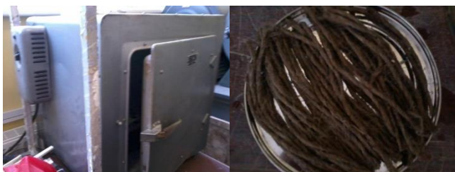
Fig. 5. The oven at 70 °C and fiber yarns on the plate
