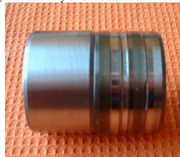
Fig. 2. New and hardly worn out shaft protective sleeve.
