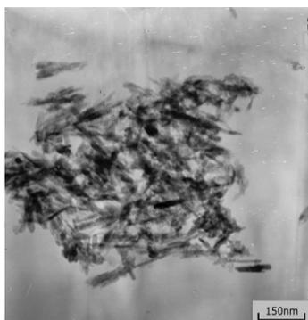
Fig. 1: The TEM micrograph of initial HAP particles
