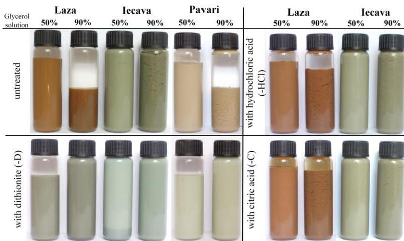
**Fig.14.** Stability of clay mineral/glycerol solution suspensions after 21 days
