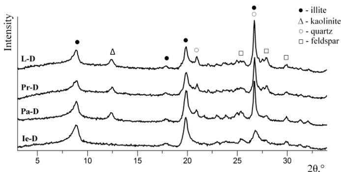
**Fig.6.** XRD pattern of clay samples after removal of iron compounds
