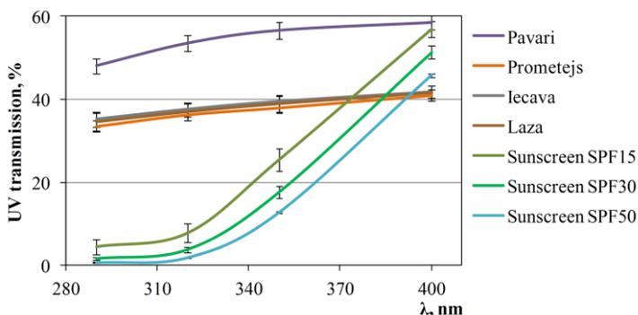
**Fig.17.** UV transmission of untreated clays with 30 wt% concentration and commercial sunscreens
