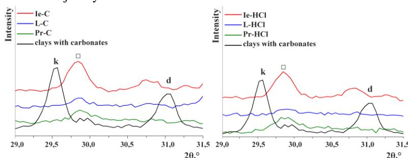
**Fig.2.** XRD pattern of clay samples before and after the removal of carbonates
