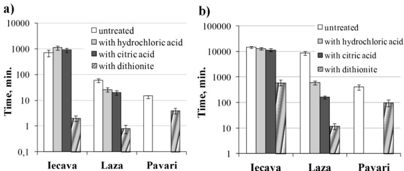
**Fig.15.** Stability of emulsions by addition of clay fractions with concentrations a) 5 wt% and b) 10 wt%
