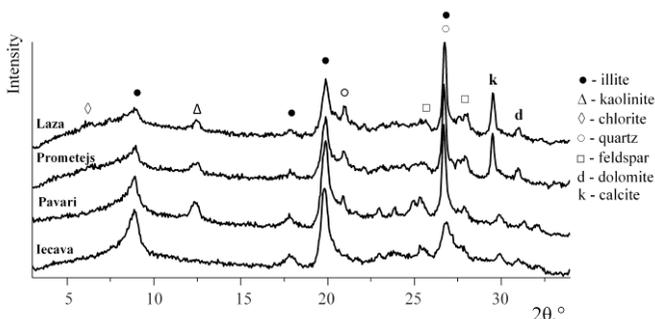
**Fig.3.** XRD pattern of untreated clay fractions
