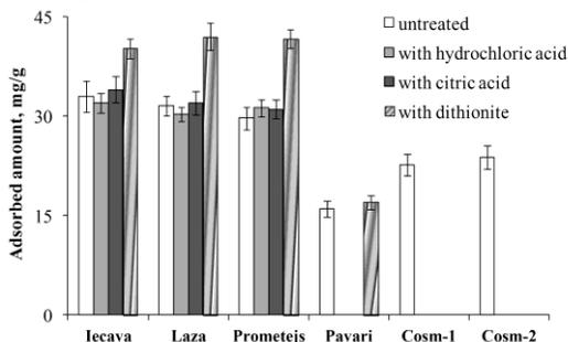
**Fig.9.** Adsorbed amount of oleic acid, mg/g
