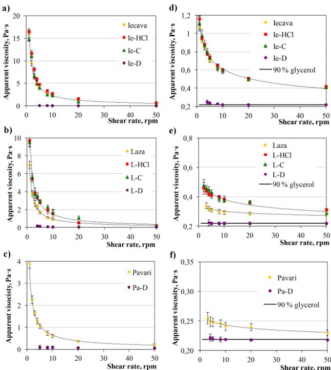
**Fig.11** Influence of the used treatment on apparent viscosity of clay suspensions in 50% glycerol solution with 20 wt% of clay fraction (a, b, c) and in 90% glycerol solution with 5 wt% of clay fraction (d, e, f)
