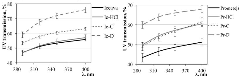
**Fig.16.** Influence of the used treatment on UV transmission of Iecava and Prometejs clays in 50% glycerol with solid concentration 20 wt%
