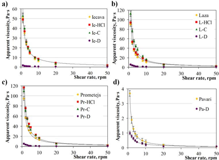
**Fig.10.** Influence of the used treatment on apparent viscosity of 50 wt% clay/water suspensions a) Iecava, b) Laza, c) Prometejs and d) Pavari clays
