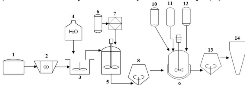
1 – untreated clays, 2 – crushing, 3 – mixing and settling tank, 4 – distilled water, 5 – vessel with mechanical mixer, gas drain and pH sensor, 6 – 1 M HCl, 7 – dispenser, 8, 13 – tube filter or rotary vacuumfilter, 9 – thermostatically controlled reactor with mechanical mixer, 10 – 3 M sodium citrate, 11 – 1 M NaHCO<sub>3</sub>, 12 – sodium dithionite, 14 – fluid bed dryer
