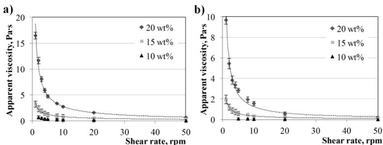
**Fig.13.** Influence of sample a) Ie-HCl and b) L-HCl concentration on the apparent viscosity of suspensions in 50% glycerol solution
