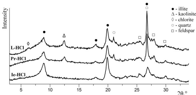
**Fig.4.** XRD pattern of clay samples after dissolution of carbonates with HCl
