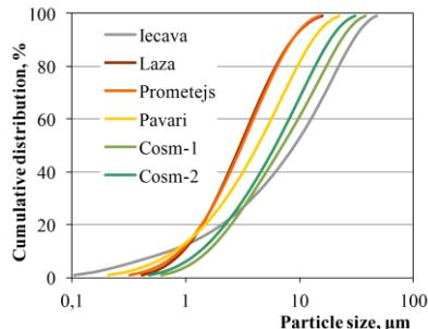
**Fig.7.** Particle size distribution of untreated and cosmetic clays
