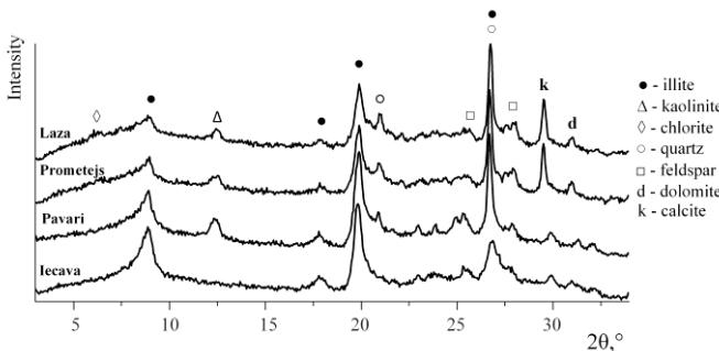
**Fig.3.** XRD pattern of untreated clay fractions
