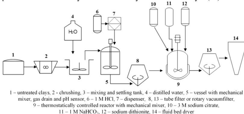
**Fig.19.** Technological sheme of clay preparation for application as sorbents in purifying masks
