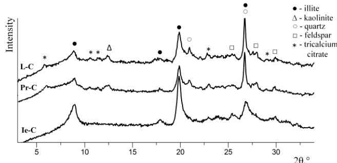
**Fig.5.** XRD pattern of clay samples after dissolution of carbonates with citric acid
