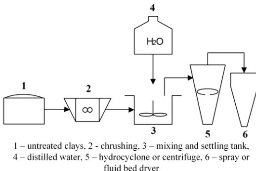
**Fig.18.** Technological sheme of clay preparation for application as UV filters
