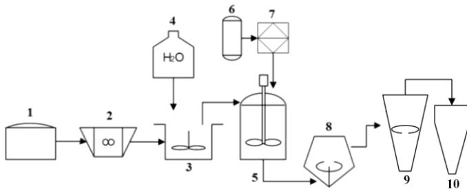
1 – untreated clays, 2 - crushing, 3 – mixing and settling tank, 4 – distilled water, 5 – vessel with mechanical mixer, gas drain and pH sensor, 6 – 1 M HCl, 7 – dispenser, 8 – tube filter or rotary vacuumfilter, 9 – hydrocyclone or centrifuge , 10 – fluid bed dryer
