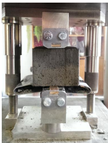
Fig. 2. Tensile split test in progress.
