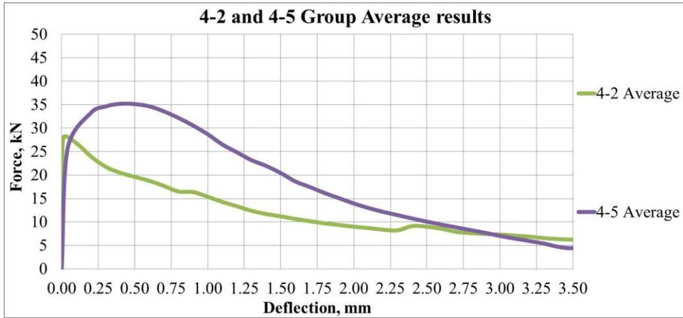
Fig. 13 Load — vertical deflection experimental graphs for specimens Group 4-2 and 4-5
