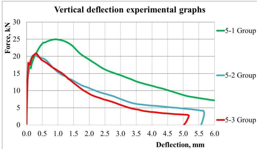
Fig. 21 Load — vertical deflection experimental graphs for specimens all Groups 0–6 mm
