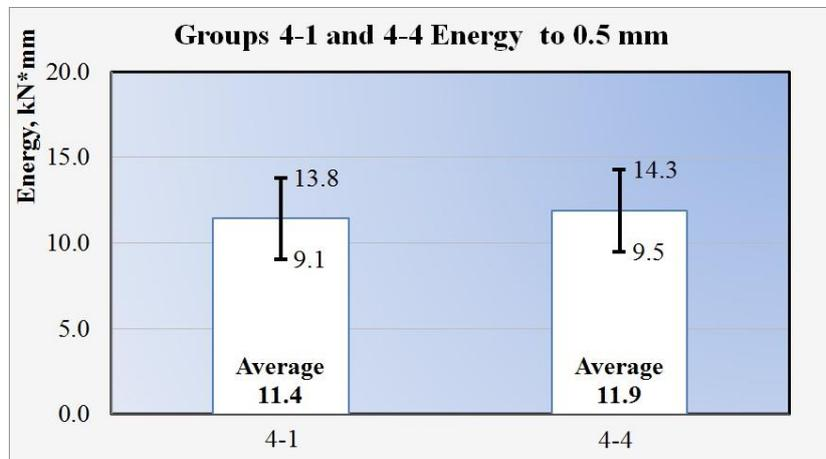
Fig. 11 Deformation energy and confidence limit Groups 4-1 – 4-4 to 0.5 mm
