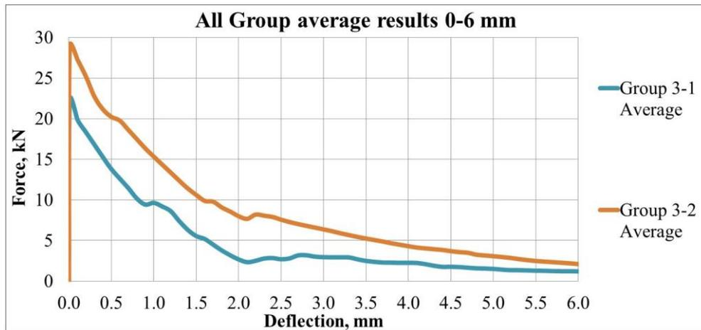
Fig. 7 Load — vertical deflection experimental graphs for specimens Group 3-1 and 3-2
