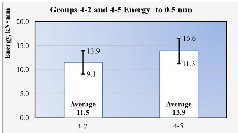
Fig. 14 Deformation energy and confidence limit Groups 4-2 – 4-5 to 0.5 mm
