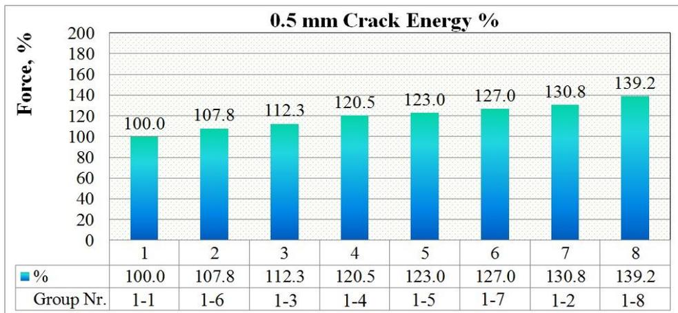
Fig. 3 Percentage of deformation energy
