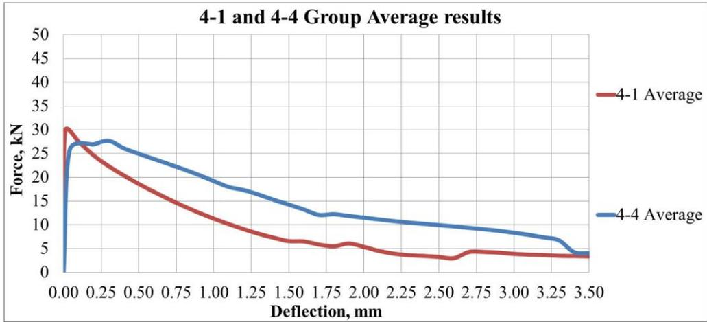
Fig. 10 Load — vertical deflection experimental graphs for specimens Group 4-1 and 4-4
