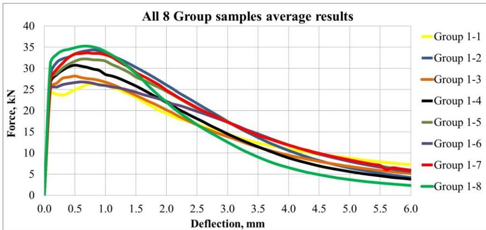
Fig. 1 Force and displacement average results for Groups 1-1 to 1-8
