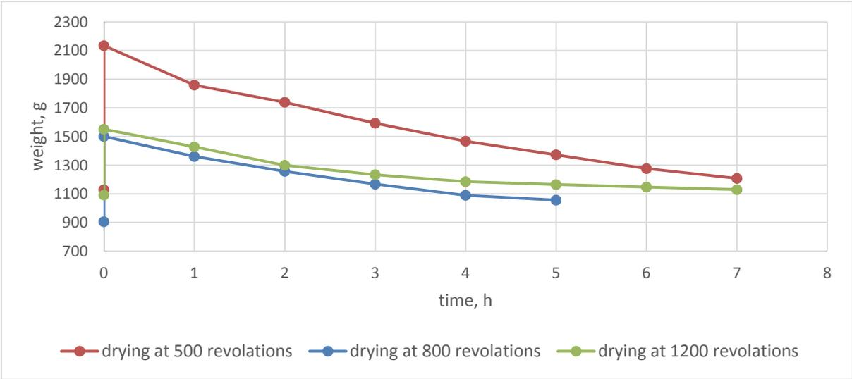
Fig. 3-4: Change in weight of clothes after washing in the automatic washing machine and indoor drying process.
