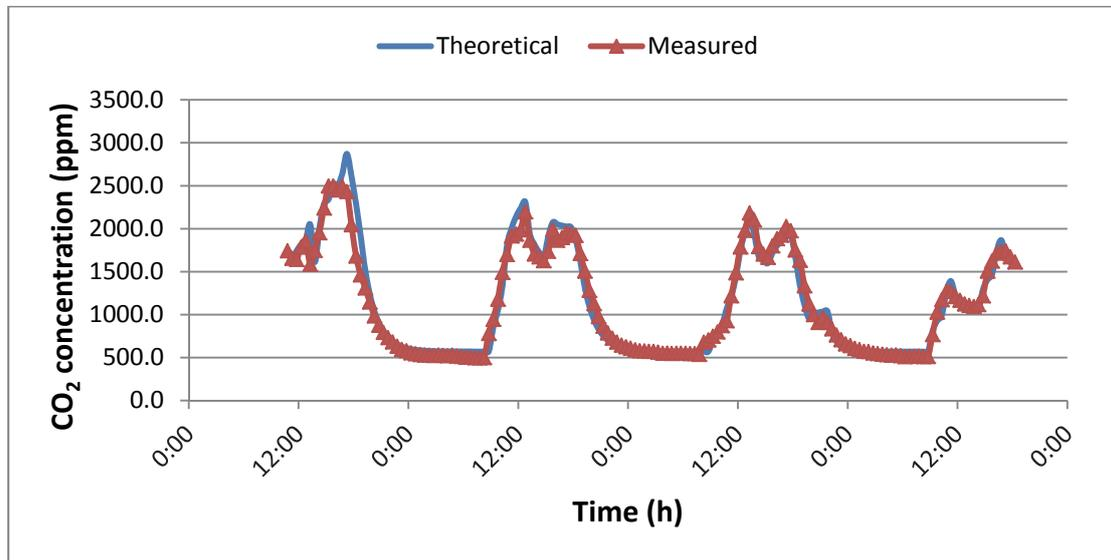
Fig. 3-1: The predicted and measured CO<sub>2</sub> concentration in the office room.
