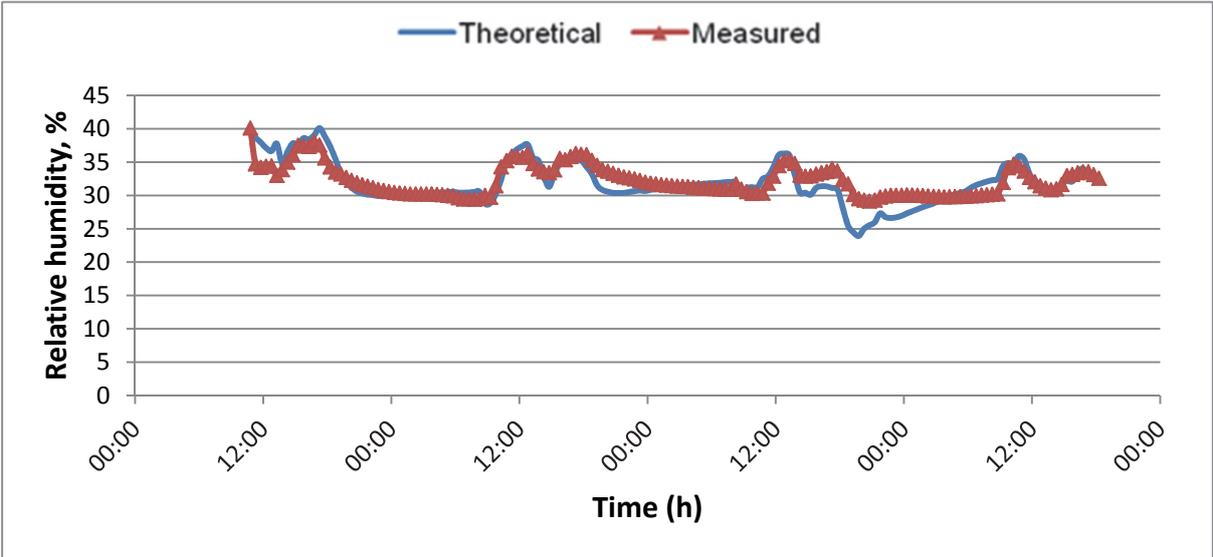
Fig. 3-6: The predicted and measured relative humidity in the office, including moisture buffering
