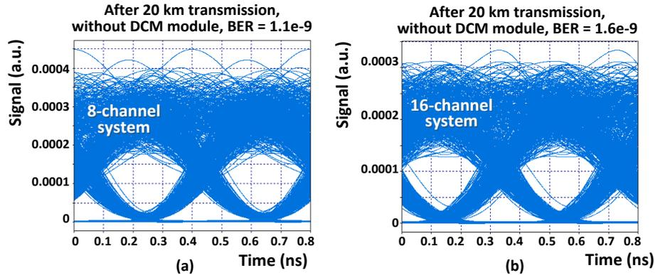
Fig. 13. Eye diagrams and BER values of received signals after 20 km transmission without use of DCM module in (a) 8-channel and (b) 16-channel 2.5 Gbit/s SS-WDM PON systems.
