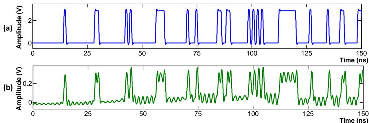
Fig. 31. (a) Time diagram of initial input electrical signal before realization of slicing operation and (b) time diagram of transmitted and restored sliced signal.
