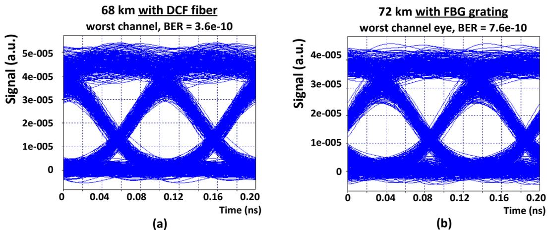
Fig. 5. Eye diagrams of received signal at maximum achieved distance in WDM-PON system by realizing CD compensation with (a) DCF DCM and (b) FBG DCM.
