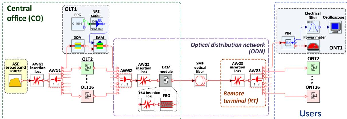
Fig. 16. Simulation scheme of 16-channel SS-WDM PON system with EAM modulator, intensity noise suppression with SOA and dispersion compensation module (DCM).
