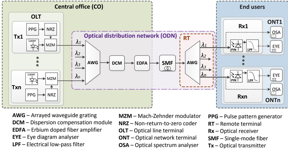
Fig. 6. Experimental model of WDM-PON optical access system with data transmission speed 10 Gbit/s per channel.
