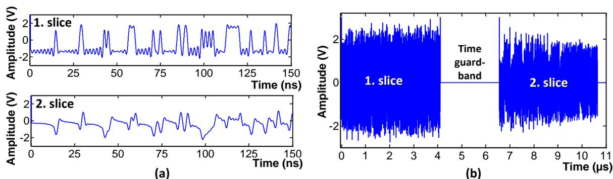
Fig. 27. (a) Separately shown time diagrams of both 500 MHz slices and (b) time diagram of formed electrical signal obtained by combining both slices in time, which is used for direct modulation of DFB laser.
