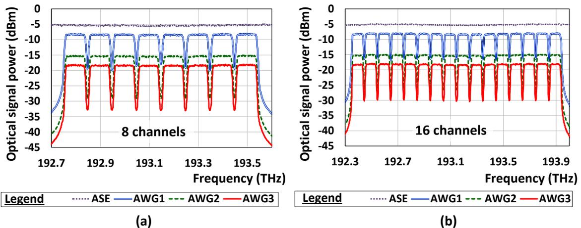
Fig. 12. Optical output spectrum of broadband ASE light source and each AWG unit in (a) 8-channel and (b) 16-channel SS-WDM PON system with line length equal to 10 km.
