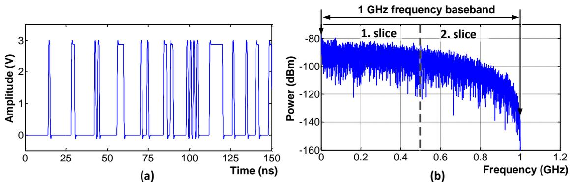
Fig. 25. (a) Time diagram and (b) spectrum of generated 1 Gbit/s electrical signal.
