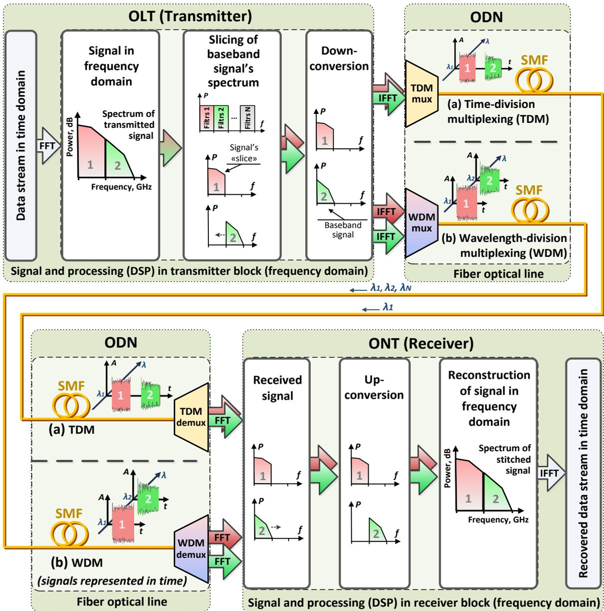
Fig. 23. Principle of slicing an input electrical baseband signal into two equal bandwidth slices at the OLT, transmission, reception and a reconstruction of the origin signal waveform at the ONT by using: (a) TDM or (b) WDM multiplexing technique.
