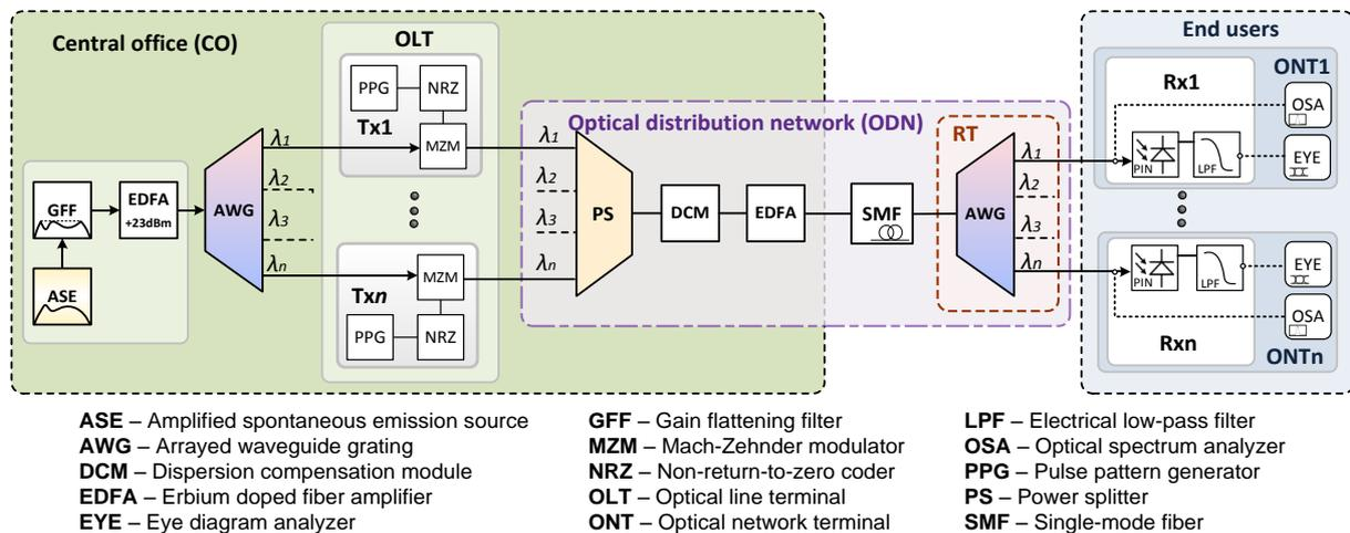
Fig. 20. Scheme of experimental up to 16-channel SS-WDM PON transmission system with data rate 2.5 Gbit/s per channel.
