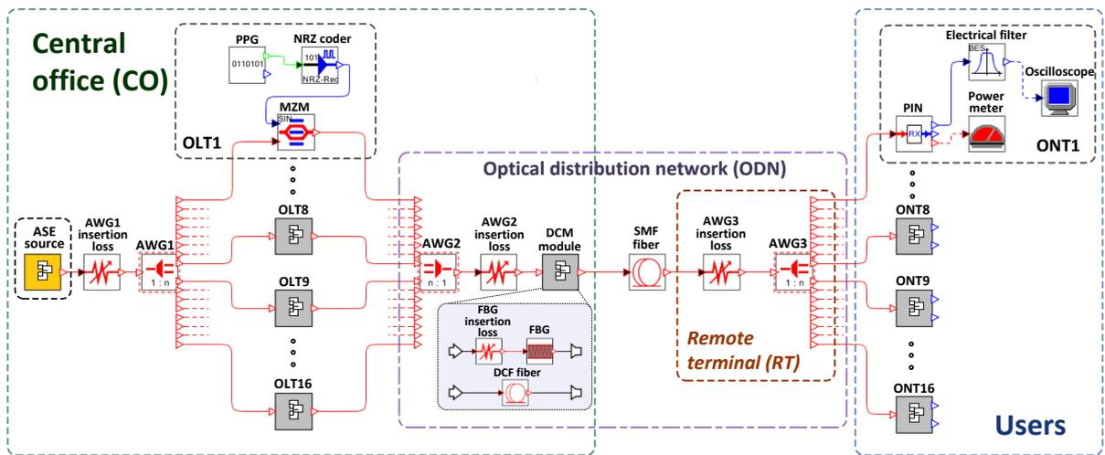
Fig. 11. Simulation scheme of up to 16-channel SS-WDM PON system with spectrally sliced broadband ASE light source and dispersion compensation module (DCM).
