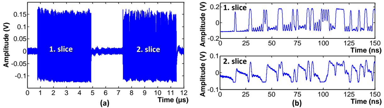
Fig. 28. (a) DSO captured electrical waveform which is used for further processing in DSP block and (b) both electrical slices of received signal, separated in time by using DSP.
