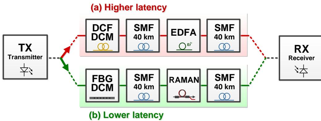
Fig. 33. Point-to-point optical metro-access network with (a) high latency conventional elements and (b) low latency optical and electro-optical elements.
