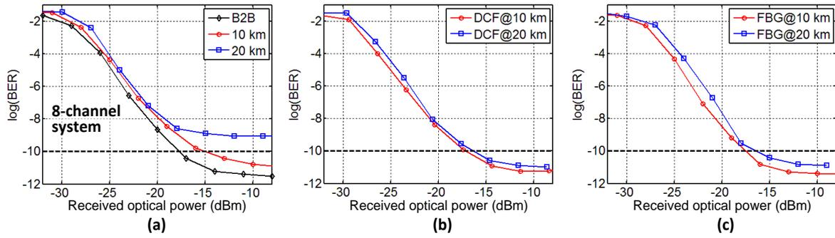
Fig. 14. BER as a function of received power in 8-channel SS-WDM PON system with various transmission distances and (a) without use of CD compensation and with implementation of CD compensation by (a) DCF fiber or (c) FBG grating.
