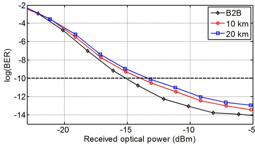
Fig. 19. BER as a function of received power in 16-channel SS-WDM PON system in B2B configuration and after transmission through 10 and 20 km long optical fiber lines.
