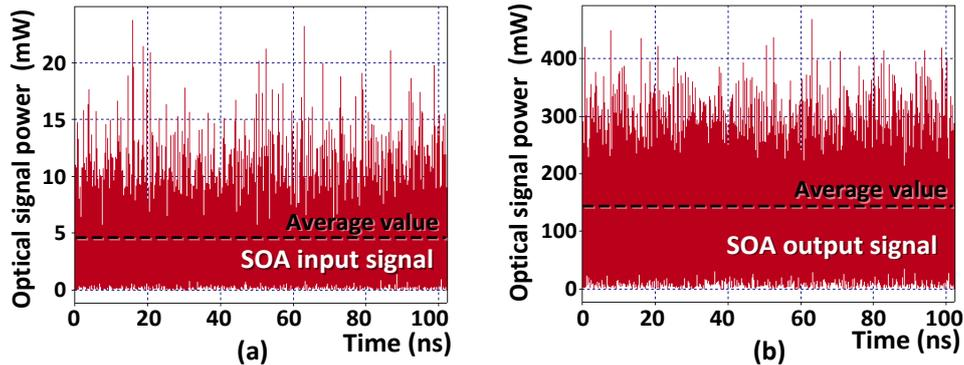
Fig. 17. Signal in time domain (a) on the input of SOA and (b) on the output of SOA after amplification and noise suppression.
