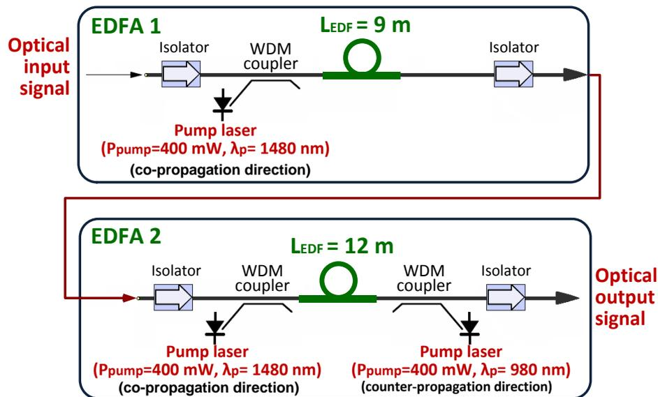
Fig. 9. Setup of two cascaded EDFA amplifiers and their basic parameters used for development of broadband ASE light source for 16-channel SS-WDM PON system.
