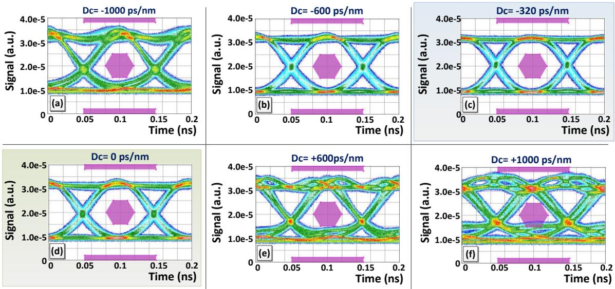
Fig. 7. Eye diagrams obtained from the worst channel of 10 Gbit/s WDM-PON access system under different FBG DCM chromatic dispersion compensation levels ( $D_c$ ): (a-b) dispersion over-compensation, (c) full dispersion compensation, (d) dispersion is not compensated and (e-f) additional amount of dispersion is added to the optical line.
