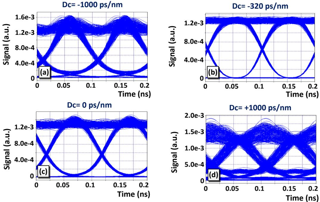
Fig. 8. Eye diagrams of received signal after 20 km transmission obtained via simulation of 10 Gbit/s WDM-PON system with different chromatic dispersion compensation values of FBG DCM module.
