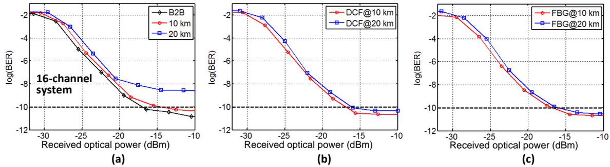
Fig. 15. BER as a function of received power in 16-channel SS-WDM PON system with various transmission distances and (a) without use of CD compensation and with implementation of CD compensation by (a) DCF fiber or (c) FBG grating.
