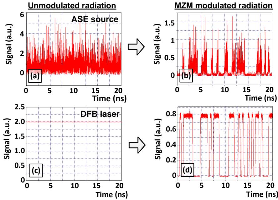
Fig. 21. Optical signal in time domain: (a) optical signal of sliced ASE light source (optical slice) in the input of MZM modulator and (b) on the output of MZM modulator after modulation; (c) radiation of DFB laser and (d) laser radiation after modulation with MZM.
