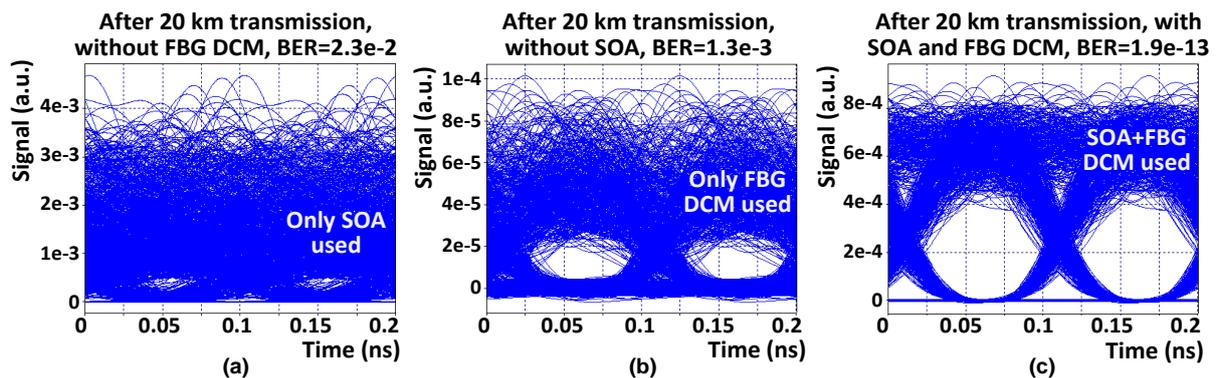
Fig. 18. Eye diagrams of received optical signals after 20 km transmission in 16-channel SS-WDM PON system: (a) without implementation of CD compensation, (b) without the use of SOA in OLT, and (c) with simultaneous use of SOA and FBG DCM at the transmitter side.
