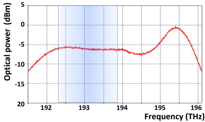
Fig. 10. The optical spectrum on the output of two cascaded EDFA system at the pump laser output power equal to  $P_{\text{pump}} = 400 \text{ mW}$ .
