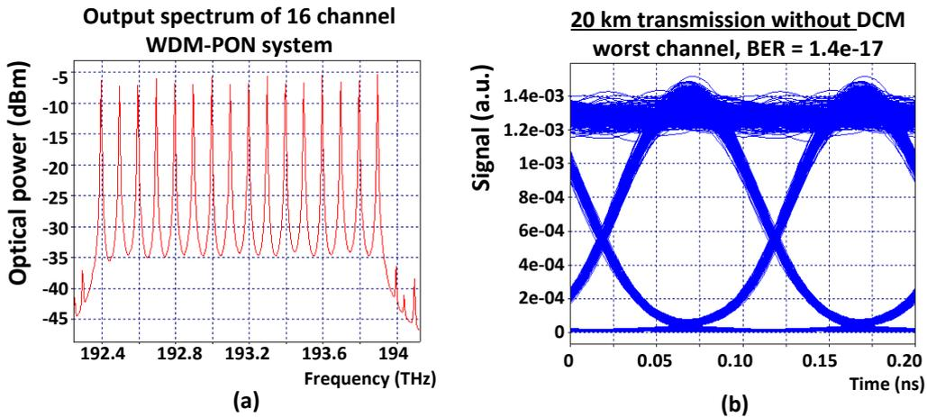
Fig. 4. Realized WDM-PON system's (a) 16-channel output spectrum after AWG demultiplexer and (b) eye diagram of the worst channel, without use of CD compensation.
