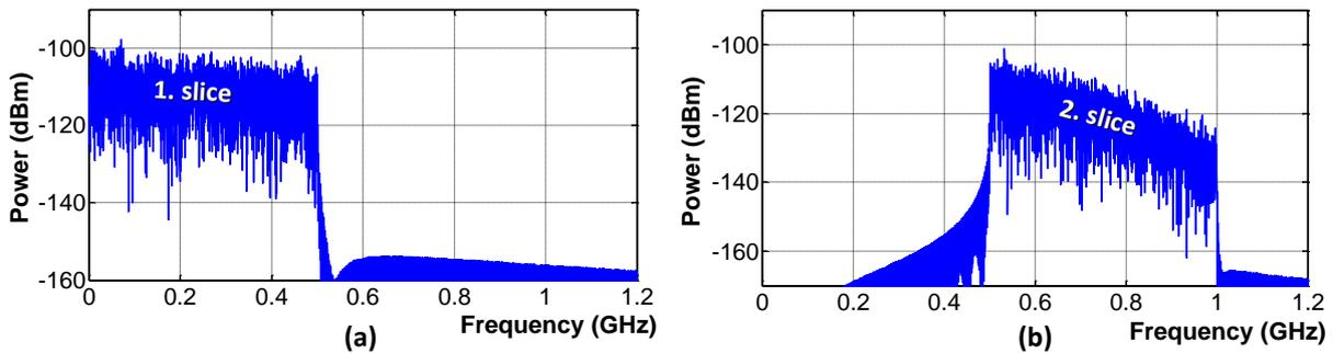
Fig. 29. (a) Spectrum of first slice and (b) second slice extracted from received signal, before realization of signal stitching operation in DSP block.
