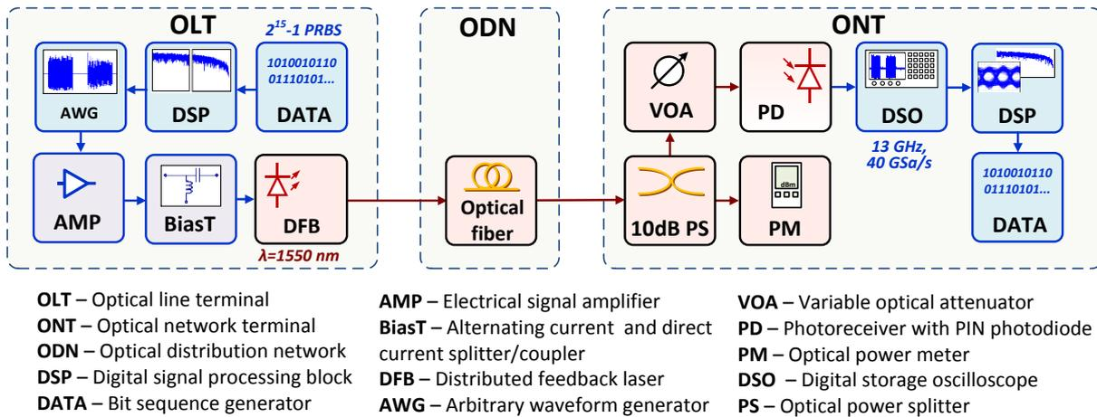
Fig. 24. Experimental setup of sliceable transceiver for slicing electrical baseband signal into two slices, transmission and reconstruction of initial signal in the receiver.
