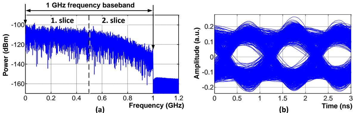
Fig. 30. (a) Spectrum of restored 1 Gbit/s electrical baseband signal and (b) its eye diagram after signal detection in B2B configuration (without using transmission line).
