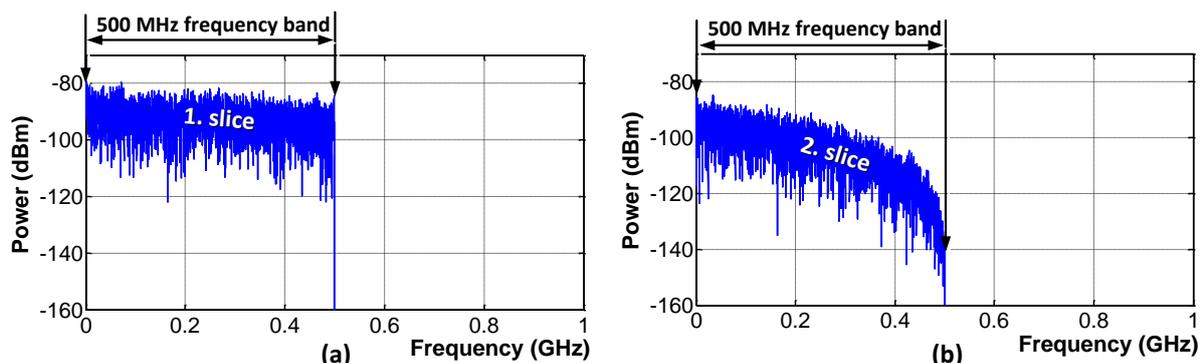
Fig. 26. Spectrum of sliced signal with 1 GHz bandwidth into two 500 MHz bandwidth slices.
