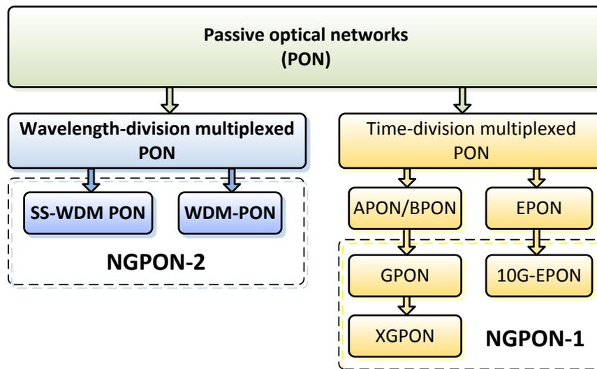
Fig. 2. Classification of passive optical access networks (PON).
