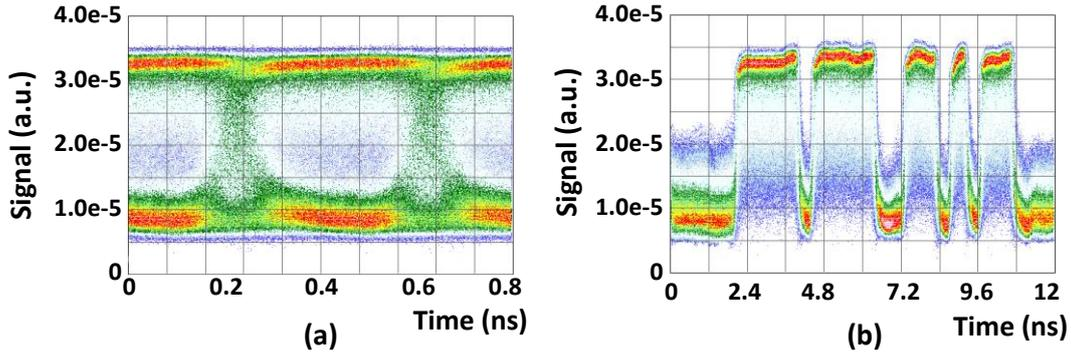
Fig. 22. Experimentally received signal's (a) eye diagram and (b) representation of signal in time domain after transmission through 10 km long optical fiber line.
