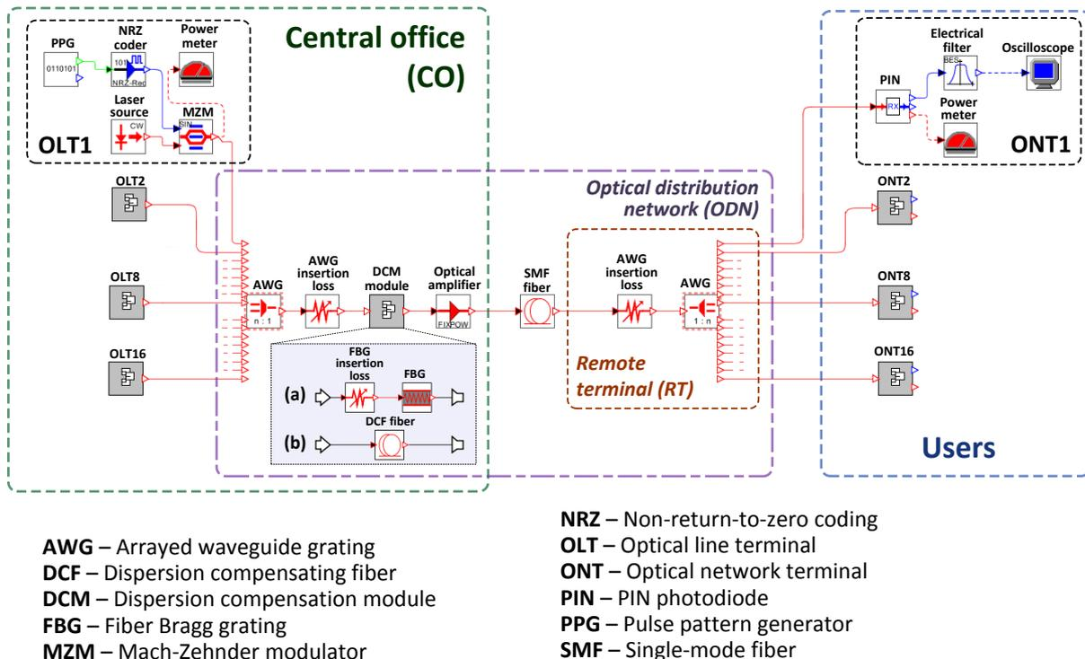
Fig. 3. Simulation scheme of dense 16-channel WDM-PON access system with NRZ coding, 10 Gbit/s transmission speed per channel and DCM module located in central office (CO).
