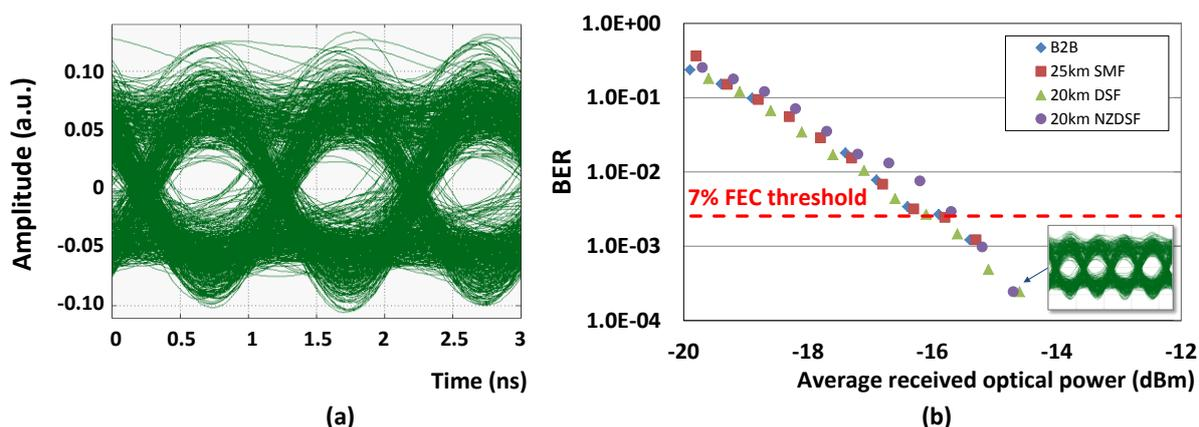
Fig. 32. (a) Eye diagram of detected and restored signal after transmission through 25 km long standard single-mode fiber, and (b) BER as a function of received power by using various optical fiber types in transmission.
