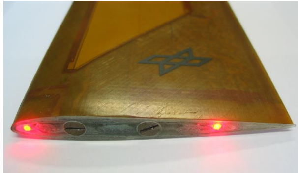
Figure 5.16. LEDs position demonstrator blade
