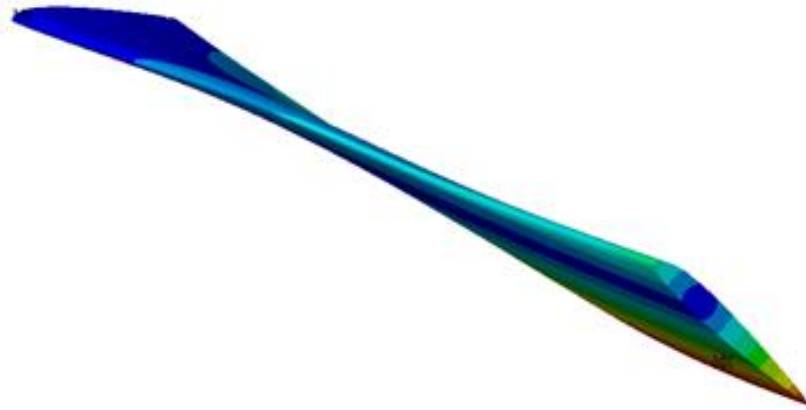
Figure 3.8. First torsion eigenfrequency of the rotor blade
