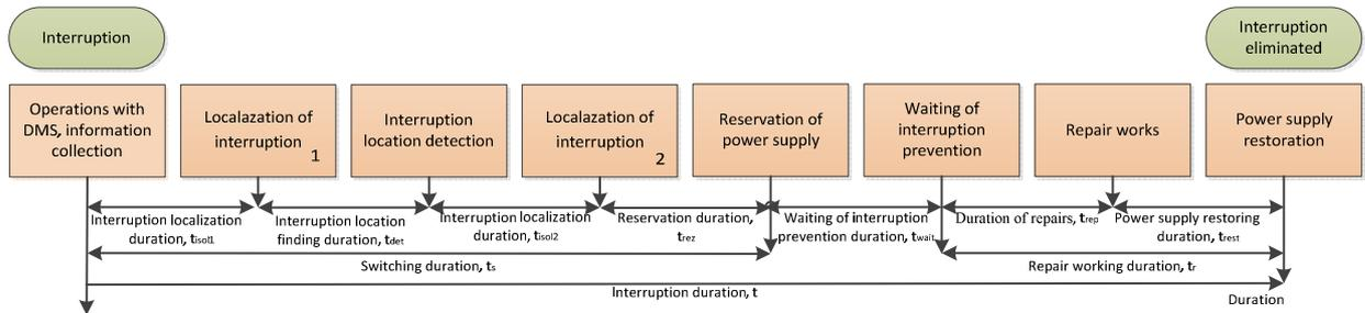
Fig. 2.2. Scale of the duration of electric supply system interruption elimination
