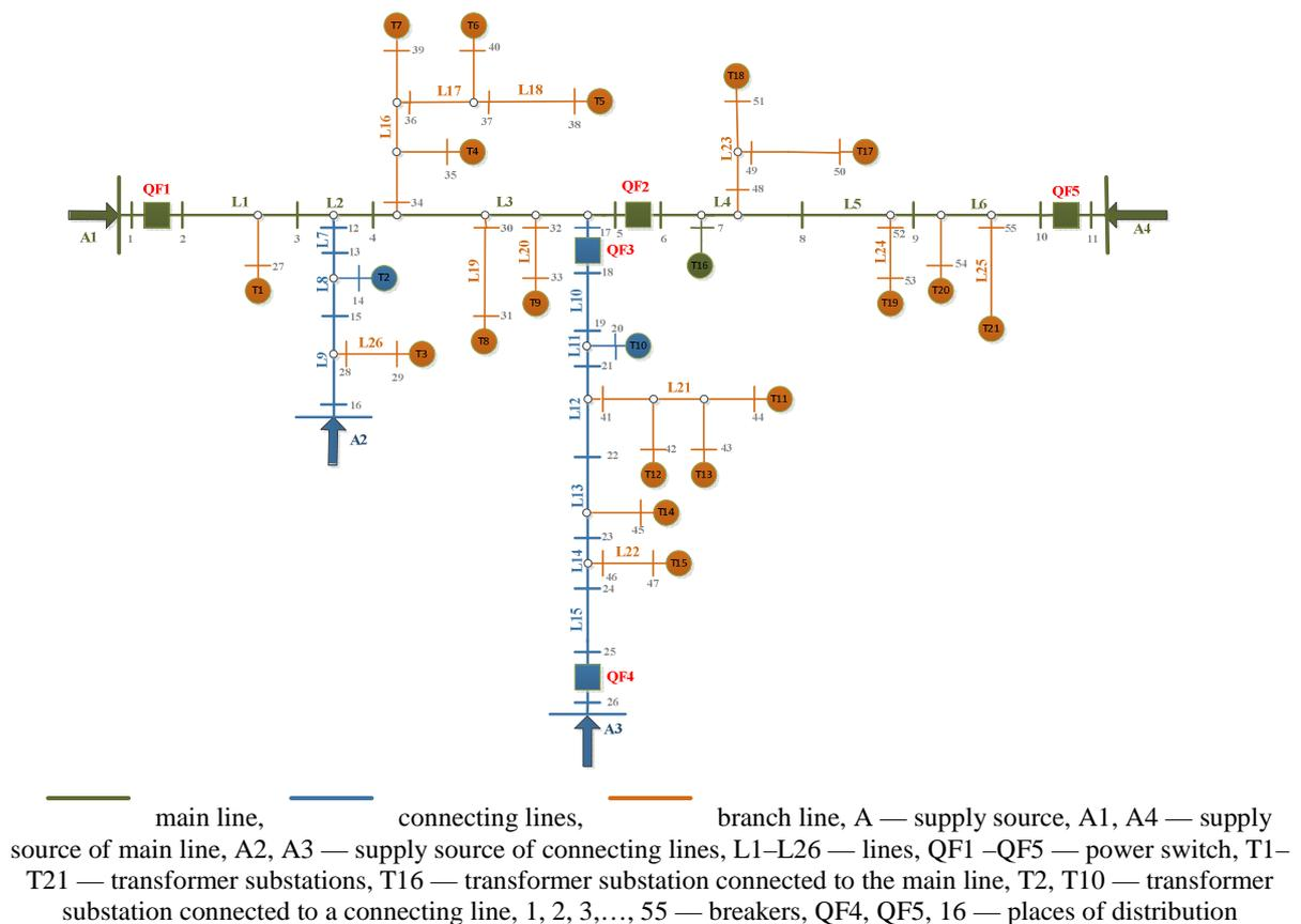
Fig. 3.2. 20 kV Model of 20 kV distribution system
