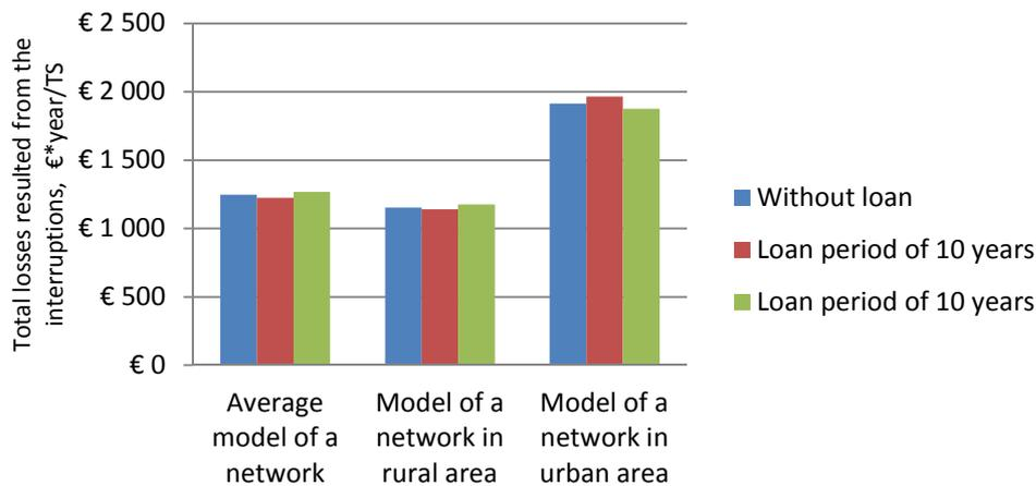
Fig. 5.4. Total losses resulting from the interruption for the case of breaker optimisation
