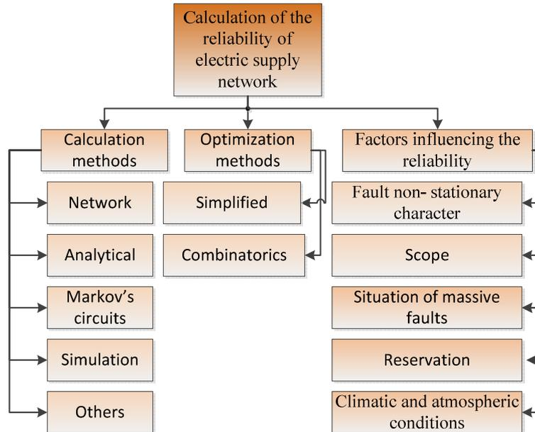
Fig. 1.1. Classification of electric supply reliability calculation methods
