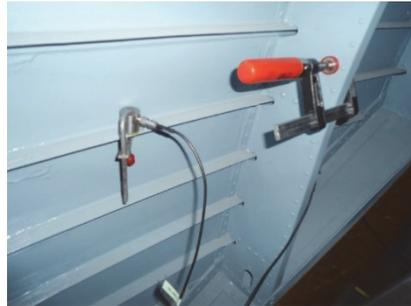
Fig. 5.2. Location of AE sensors on helicopter fuselage.
