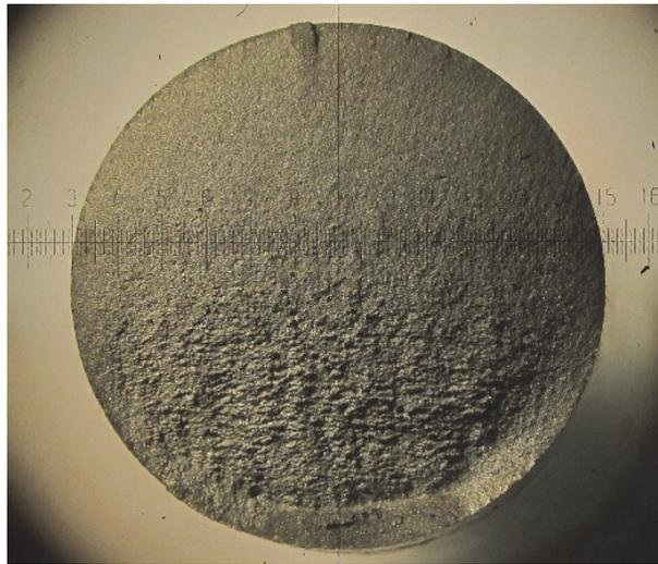
Fig. 5.16. Fracture of bolt No. 19-3 on the bolt shank.
