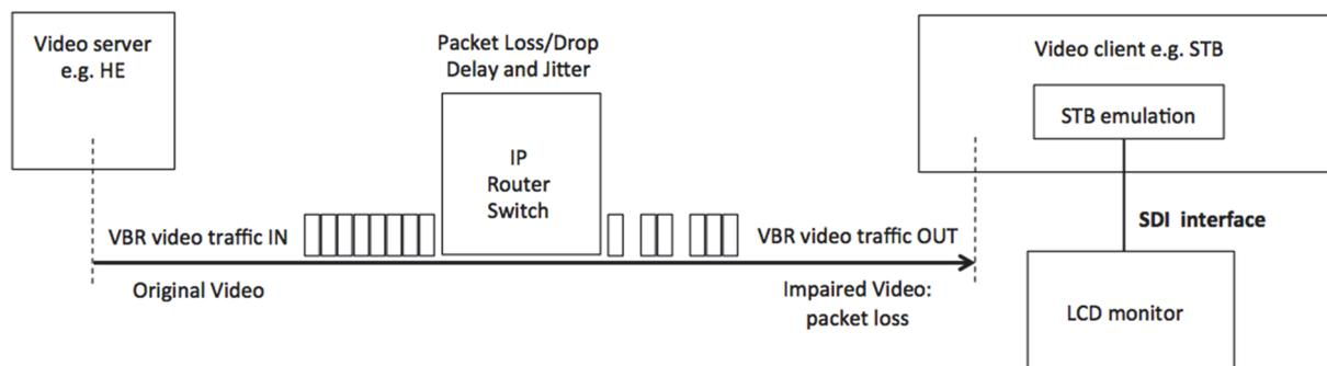
Fig. 3.2. The block diagram of video broadcasting channel quality assessment.
