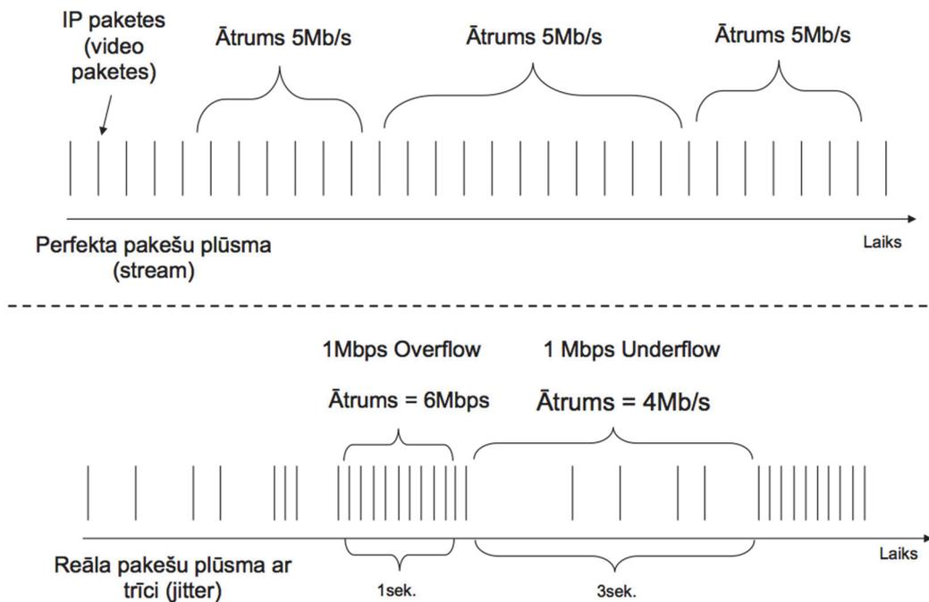
Fig. 1.1. Packet broadcasting process with delays and jitter.
