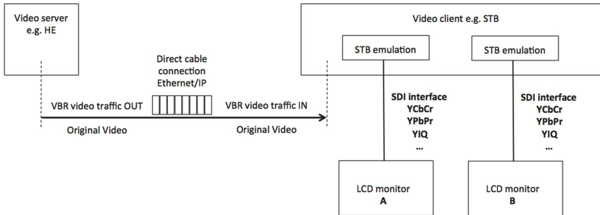
Fig. 3.1. The block diagram of video coding quality assessment.
