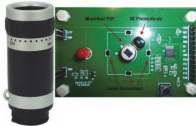
Fig. 61 Hybrid sensor board and off the shelf zoom 8X Field 9°
