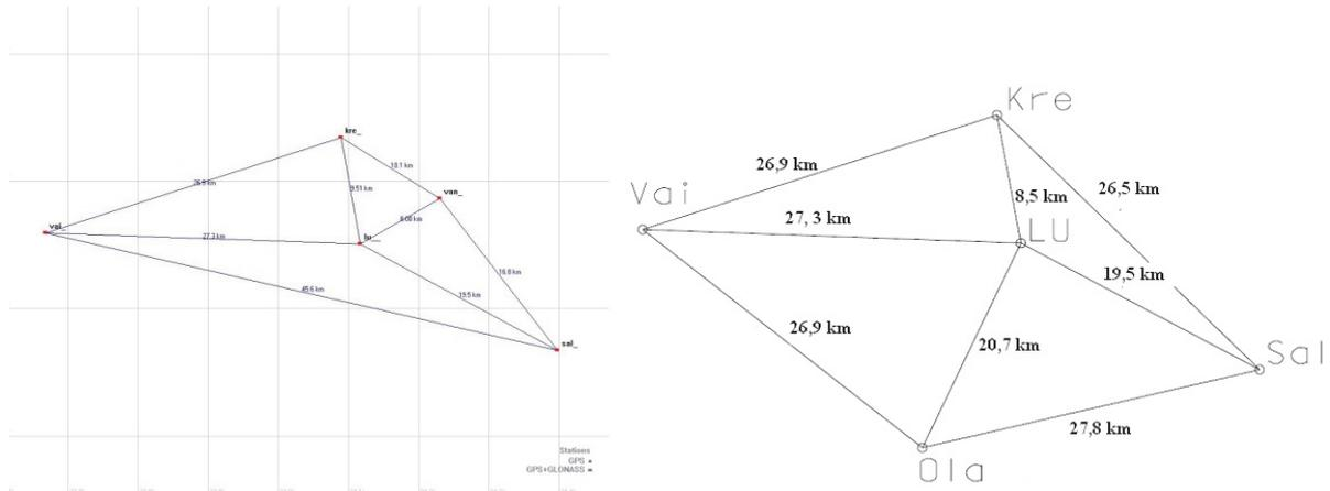
**Fig. 3.7.** Existing (to the left) and proposed (to the right) base station geometric location for homogeneity improvement.
