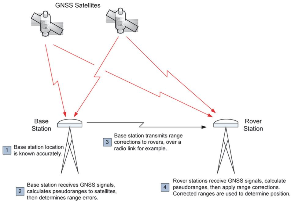
**Fig. 1.1.** Typical reference system principles.
