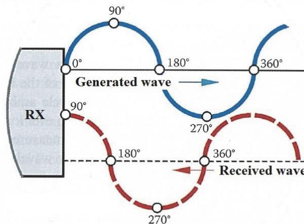
**Fig. 2.1.** Phase shift of generated and received wave.
