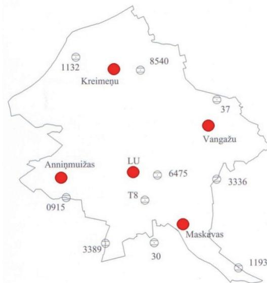
**Fig. 3.1.** Used RG2 points for accuracy evaluation of measurements (red – original *EUPOS®-RIGA* base station location).
