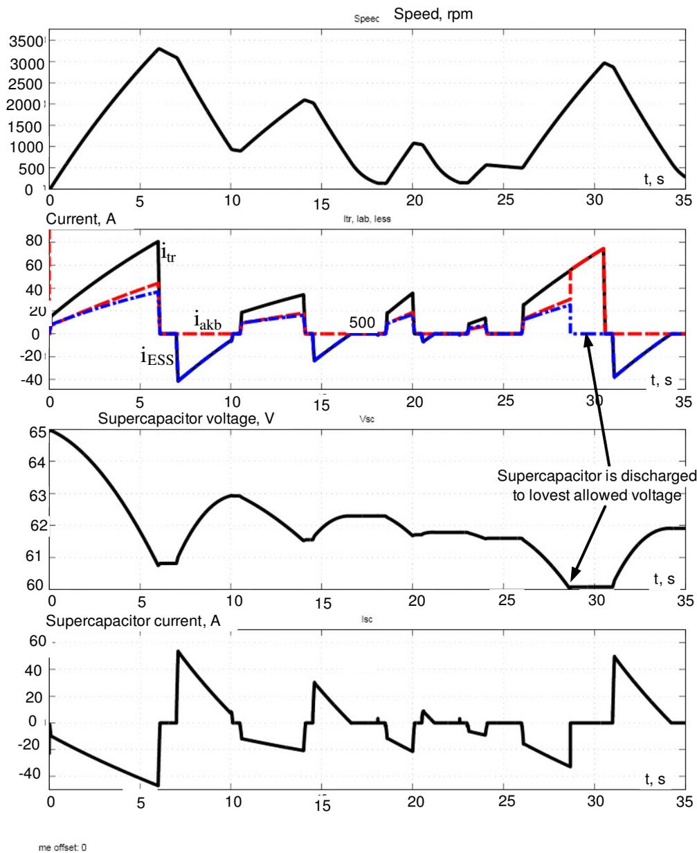
**Fig. 4. Current and voltages waveforms at the ESS converter proportional control algorithm**
