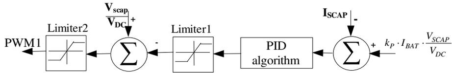
Fig. 7. Control algorithm of the converter in boost (discharge) mode
