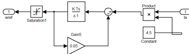
Fig. 3. Controller of the load simulator
