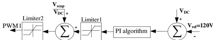
Fig. 9. Control algorithm of the converter in buck (charge) mode
