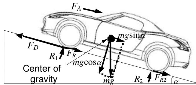
Fig. 2. Forces acting on a vehicle
