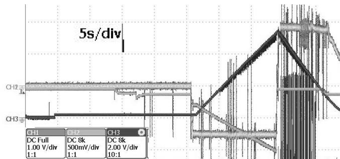
Fig. 6. Emulation of the real LEV on the test bench: CH1 – motor current 100 mV = 1 A (inverse); CH2 – battery current 100 mV = 1 A (inverse); CH3 – signal proportional to the speed
