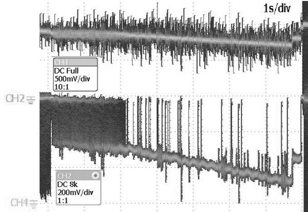
Fig. 8. Control of the ESS current proportionally to the battery current in discharge mode:
