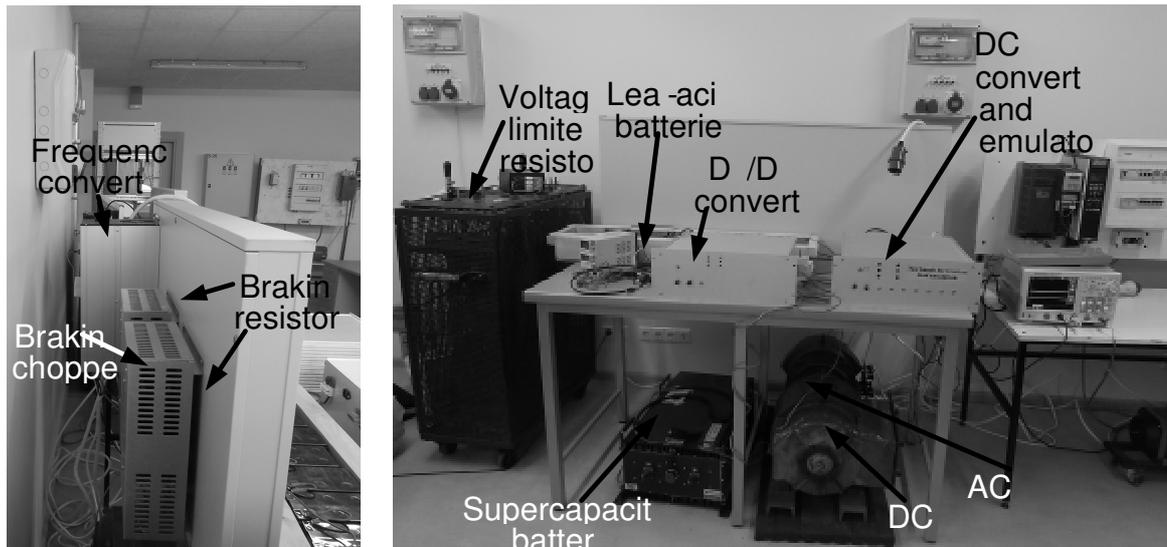
Fig. 5. Test bench used for proportional control algorithm examination
