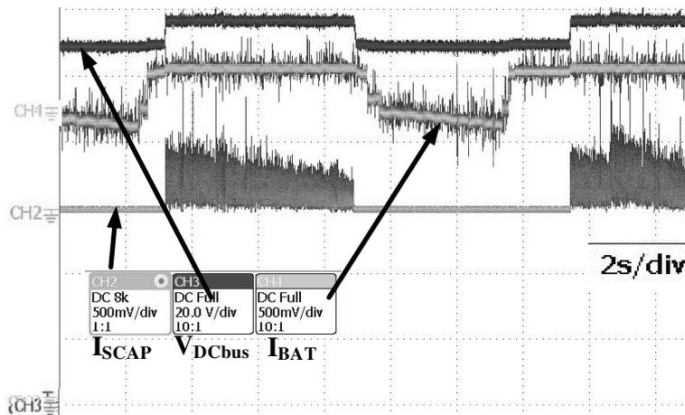
Fig. 10. Control of the ESS in the braking mode: before PID control loop tuning and after tuning
